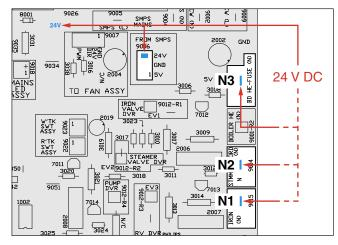
To check 5 V DC : <sup>1)</sup> Probe at 5 V test point and N1/N2/N3. or <sup>2)</sup> Probe at connector 9019 between VDD and GND
