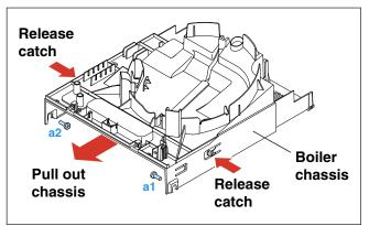
Pull outCHASSIS BOILER ASSY 49DisassembleWIRE ASSY LED - RINSE TANK 40DisassembleWIRE ASSY RINSE TANK SWITCH 42DisassemblePUMP ASSY 50DisassembleELECTROVALVE 51
