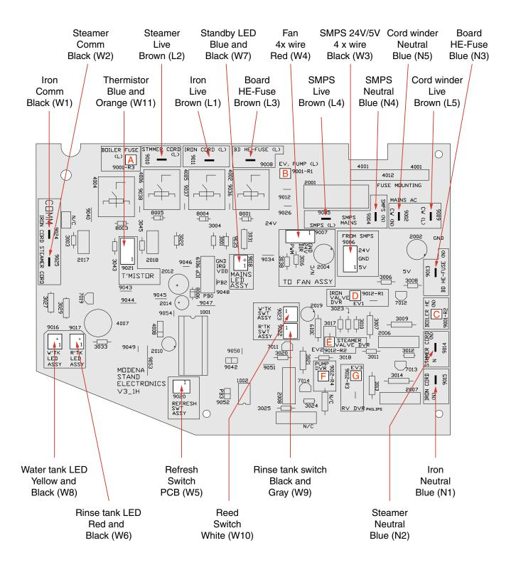
NOTE : ABC (brown, red, and blue) is a 3 pole connector to connect to boiler side. (W12) DEFG (white, blue, yellow and black) is a 4 pole conn to connect to boiler side (W13)
