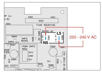
4.2 Check for output of 24 V DC and 5 V DC from switch mode power supply. To check 24 V DC : Probe at 24 V test point and N1/N2/N3.
