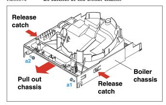
Pull out CHASSIS BOILER ASSY 23
