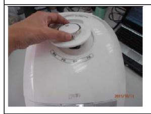
2、separate steam valve cover from steam valve base
