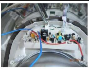
21, pull up flat cable of display board.
