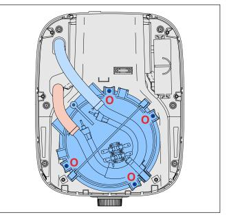
Step 6: Grinder, Synchro motor and Water supply To remove the Grinder, disconnect its leads from the main PCBA and undo screws (U). To remove the Synchro motor remove its leads from the main PCBA and undo screws (♥). The top water supply, consisting of the shower head, silicon hose, elbow and riser pipe, can be removed by undoing screws (\$), only when the Silicon hose needs
