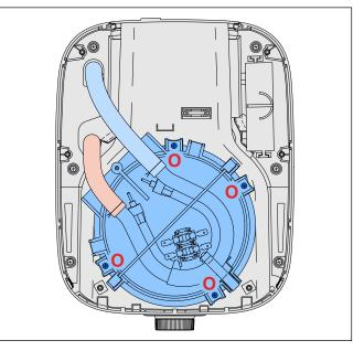
Step 6: Grinder, Synchro motor and Water supply
