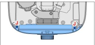
Undo the snaps by tracing the curve of the UI panel with a flat-head screwdriver, while pulling the UI panel upwards.
