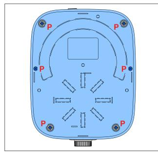
The PCBA is in the plastic box indicated in blue, some leads need to be released before you can take out the PCBA completely.
