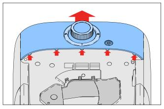
The UI panel can be disassembled, the rotary knob can simply be pulled off, the rotary encoder is secured by a single nut, remove the nut. The PCBA cover is held in place by six screws (L), once unscrewed the PCBA can be taken out. Please mind the rubber seal, preventing steam from reaching the UI PCBA.
