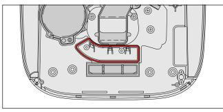
When the UI panel or Synchro motor has been removed, special attention is needed to the proper wire routing from top to bottom. All wires must pass through the slots as indicated in red in the cross section below. They may not be passed through the opening for the Grinder.
