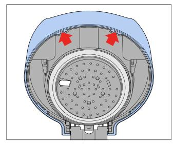
Caution, the hinge spring on the back side of the appliance may come out when the brewhead lid cover is being removed. When reinstalling it, mind your fingers as this is a strong spring.
