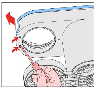
The top cover needs to be tilted forward to be removed. The flat cable **W** from the main PCBA to the UI PCBA is still attached to the User Interface panel, and can easily be unplugged.
