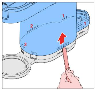
Remove the housing upwards from the rest of the appliance, but mind flat cable running through the guide on the inside of the housing and the water level sensor still connected to the inside of the housing.
