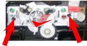
Loosen the screw and remove the control knob and coffee keys.
