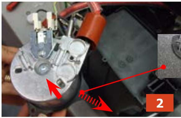
2) Loosen the screw and remove the plastic support. Disconnect the hoses and the connections.
