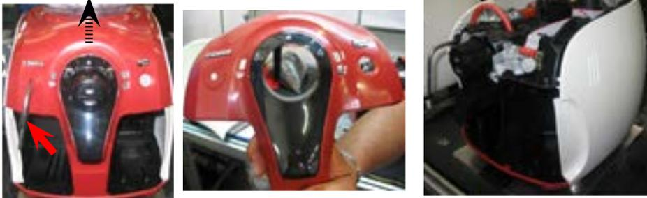
Slide out the steam hose protection, lift the cover at the rear by pressing down gently on the cooling vents to help detach the anchoring tabs, then pull it away from the steam hose, taking care not to scratch it.
