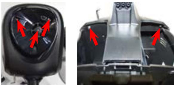
Remove the dreg drawer, water tank, mushroom finger protection device on the coffee container lid, then loosen the screws shown.
