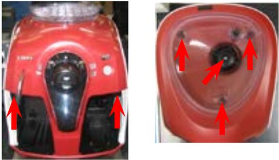
Remove the dreg drawer, water tank, mushroom finger protection device on the coffee container lid and coffee container, then loosen the screws shown.
