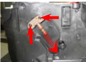
Loosen the screws shown and remove the boiler pin.
