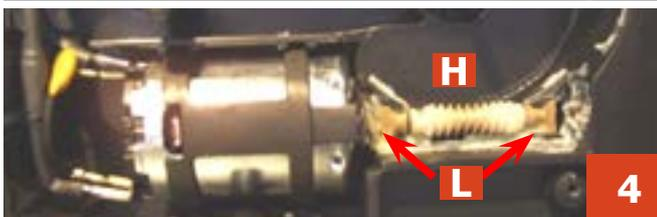
**4)** When replacing the motor and the transmission shaft, make sure the bearings (L) are in the right position.
