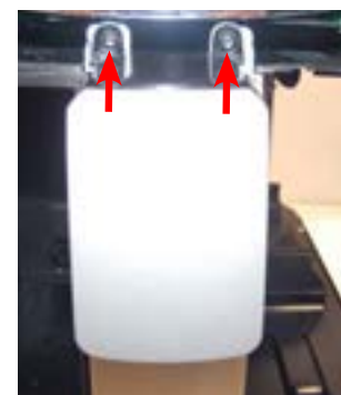
Loosen the screws as illustrated and remove the front panel to access the screws which fix the dispenser cover into place
