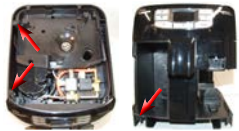
Unscrew the screws shown and slide out the left side body.
