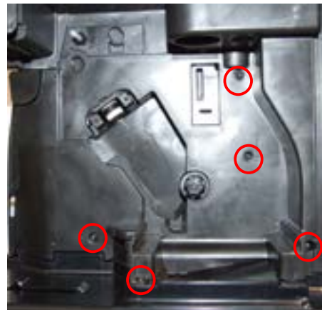
Loosen the screws as illustrated and remove the gear motor cover.
