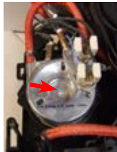
Unscrew the marked screw and disconnect the electrical and water circuit connections.
