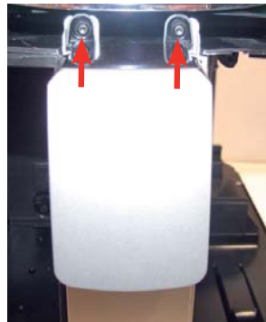
Unscrew the screws as illustrated and remove the front panel to access the screws which fix the dispenser cover into place.
