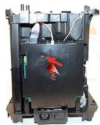
Loosen the screws as illustrated, slide out the electrical connection and remove the card guard.
