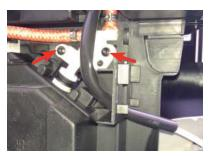
Loosen the screws as illustrated, remove the hydraulic connections and take out the valve
