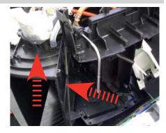
Loosen the screws as illustrated and release the insert in the bottom of the body to obtain easy access for valve disassembly
