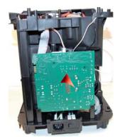
Slide the card off the support and disconnect the electrical connections.
