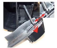
Unscrew the screws as illustrated and remove the front panel to access the screws which fix the dispenser cover into place.
