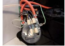
Unscrew the marked screw and disconnect the electrical and water circuit connections.
