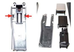
Press the hooks as illustrated and slide out the dispenser assembly.
