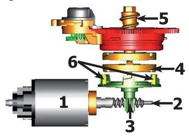
The coffee grinder is driven by a direct current motor (1) using a worm screw helicoidal wheel transmission (2).
