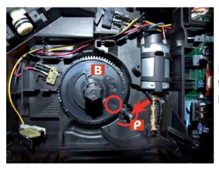
Replace the gear (B), making sure that the imprint of the arrow is aligned with the opening containing the pin (P).
