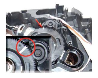
For a standard adjustment, both markings must be aligned.
