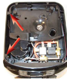
Unscrew the screws shown and slide out the left side body.
