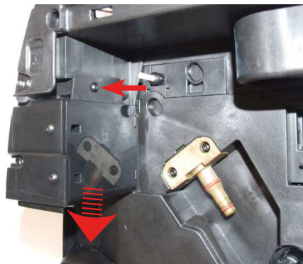
Unscrew the screws (highlighted) and release the milk jug plug body assembly
