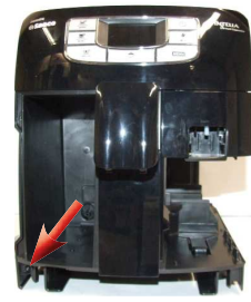
Unscrew the screws shown and slide out the left side body.
