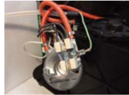
Unscrew the marked screw and disconnect the electrical and water circuit connections.
