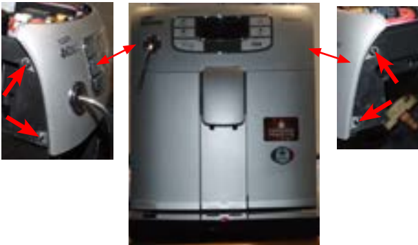
Unscrew the screws as illustrated and remove the front panel to access the screws which fix the dispenser cover into place.
