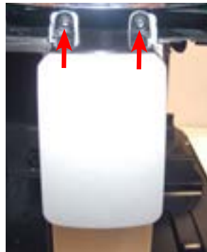
Loosen the screws as illustrated and remove the front panel to access the screws which fix the dispenser cover into place.
