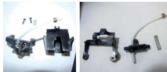
When reassembling the assembly to be careful to correctly position the spring.
