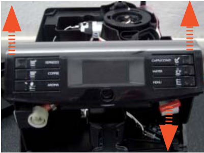
Remove the board support assembly and disconnect the electric connection
