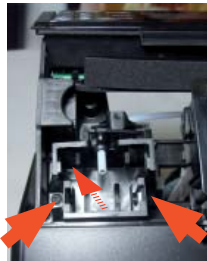
Loosen the screws holding the carafe connection
