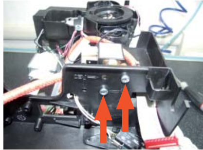
Loosen the screws holding the solenoid valve to the upper plate
