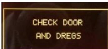
If you submit the following screen means that there is the coffee grounds drawer is not correctly inserted, or the side door is not completely closed. Only after entering the drawer and closed the door, the following screen will disappear.
