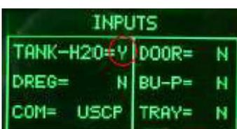
**ERROR:** The indication TANK-H2O doesn't change; check the capacitive sensor (fixing) and the wiring (JP23)
