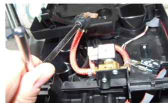
Disconnect the water circuit connection
