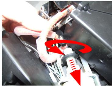
Unscrew the pump from the safety valve and slip off the pump off the upper support
