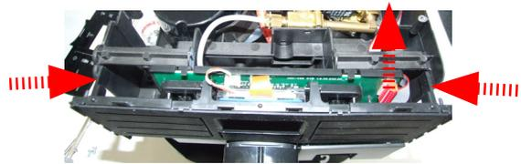
Disconnect the electrical connections. Press to right and left and lift the assembly KYB.
