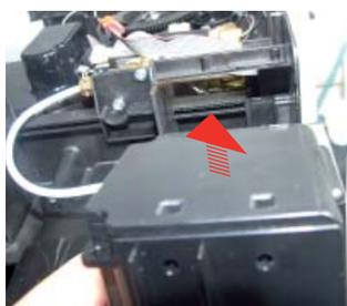
Remove the cover, loosen the screws and support teflon tube
