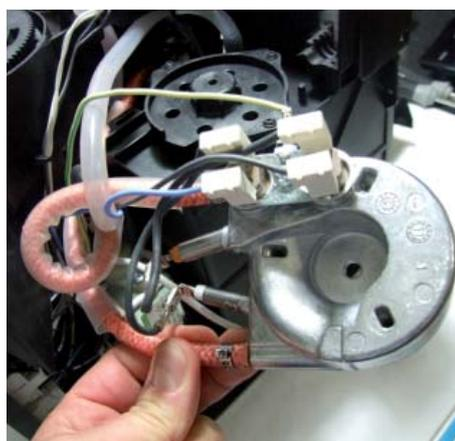
Unscrew the screw shown and remove the electrical and water circuit connections.
