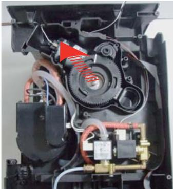
Raise the coffee grinder and remove the connections.
