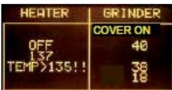
If temperature is over 135°C, the backlight change from GREEN to YELLOW. This is a ALERT message to avoid heating the HEATER element over dangerous temperature.
