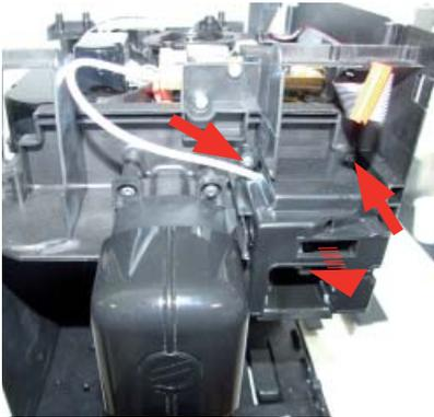
Loosen the screws and remove the assembly graft milk carafe (Moltio One Touch Milk Carafe)
