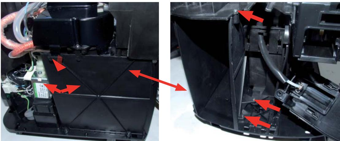
Loosen the screws as illustrated and release the insert in the bottom of the body to obtain easy access for valve disassembly
