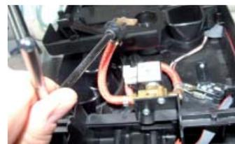
Disconnect the water circuit connection
