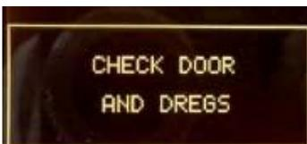
If you submit the following screen means that there is the coffee grounds drawer is not correctly inserted, or the side door is not completely closed. Only after entering the drawer and closed the door, the following screen will disappear.
