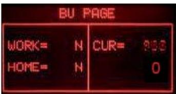
**ERROR: (Without BU)** The absorbed current is higher than 200mA, the display backlight changes from green to red; check the BU and the motor.
