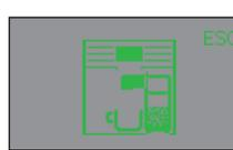
The machine will remind the user that the carafe must be inserted.
