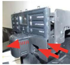
Loosen the screws and remove the cover evidenced. (Moltio One Touch Milk Carafe)
