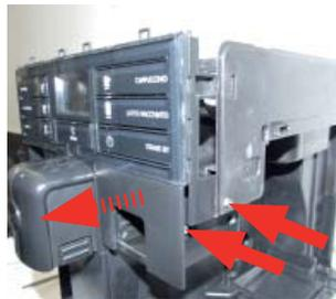
Loosen the screws and remove the cover evidenced. (Moltio One Touch Milk Carafe)
