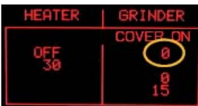
**ERROR:** The number remains 0 or the grinder does not run, the display backlight changes from green to red; check the Hall sensor board of the Grinder, the Grinder, the wiring from the Hall sensor board to the CPU/POWER board (JP2) and the wiring from the Grinder to the CPU/POWER board (JP8)
