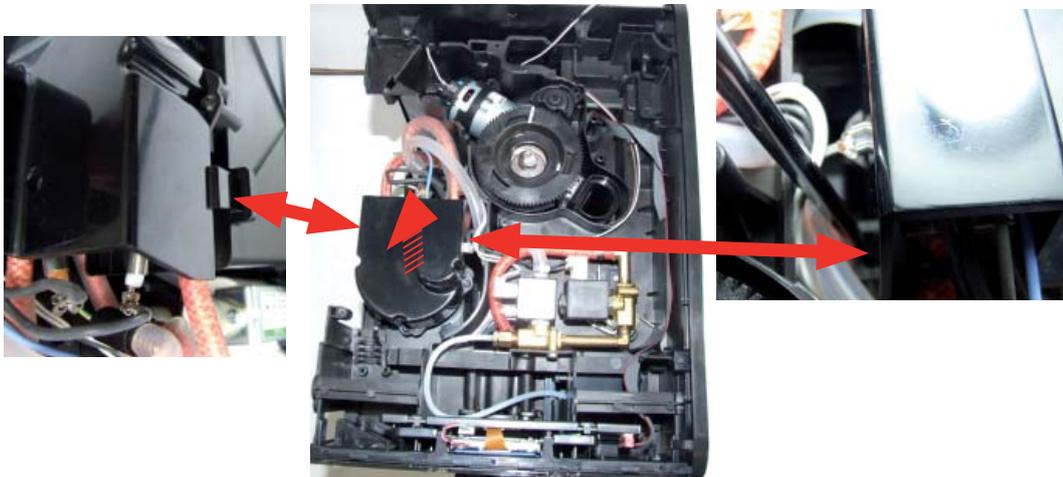
Remove the cover of the boiler by pressing the two sides with the help of a screwdriver
