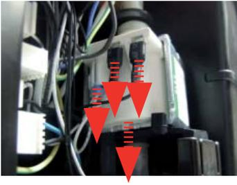
Disconnect the water circuit, electrical and remove the pump from the bottom support
