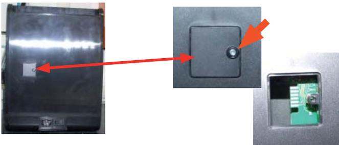
Loosen the screw for remove the cover.
