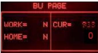
**ERROR: (With BU)** The absorbed current is more than 300mA, the display backlight changes from green to red; check the BU and the motor
