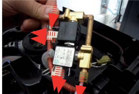
Disconnect all electrical and water circuit connections (Moltio Milk One Touch Carafe)
