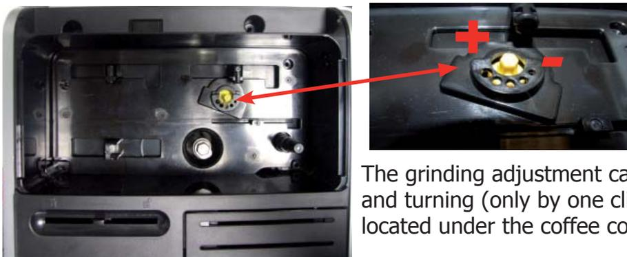
The grinding adjustment can be set by the user by pressing and turning (only by one click at a time) the insert that is located under the coffee container.
