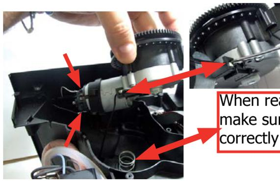
When reassembling the coffee grinder, make sure the spring is repositioned correctly (see photo).
