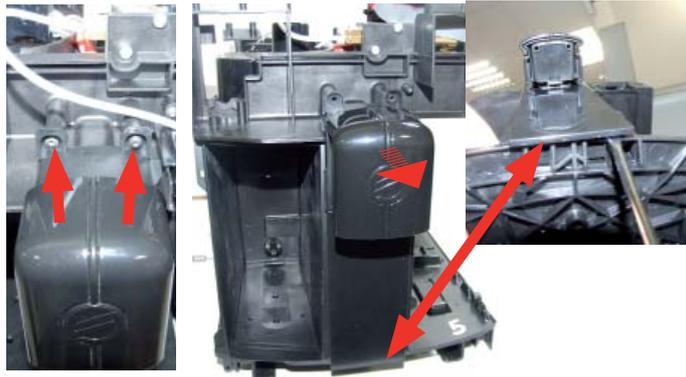
Loosen the screws and remove the assembly dispenser coffee proceeding as in the picture
