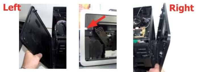
Unscrew the screw shown and remove the lateral panels
