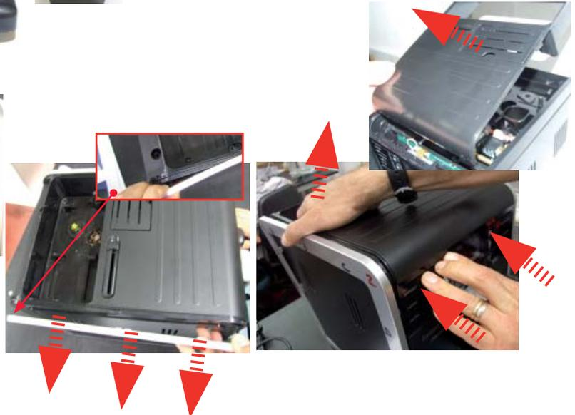
Unhook the highlighted frame and press and lift the top cover.
