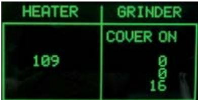
**ERROR:** if the text shown "COVER ON" / "COVER OFF" does not reflect the PRESENT / NOT PRESENT status of the Bean Hopper Cover, check the magnet presence on the cover, the REED sensor on the Bean Hopper and the REED cable to the JP25 connector onto the CPU/POWER board.
