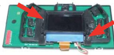
Disconnect the electrical connections evidenced.
