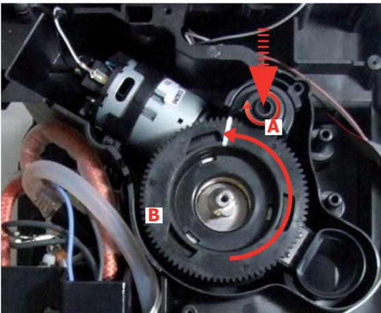
To extract the top support of the appliance, press on the grinding adjustment spindle (A) and turn the support anticlockwise until it unhooks.
