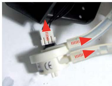
Lift the flow meter out of the casing assembly and remove the electrical and water circuit connections.
