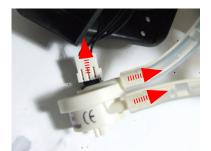
Lift the flow meter out of the casing assembly and remove the electrical and water circuit connections.
