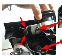
When reassembling the coffee grinder, make sure the spring is repositioned correctly (see photo).
