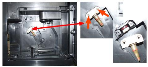
Loosen the screws as illustrated and remove the boiler pin
