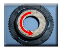
Turn the grinder blades clockwise out of the support. The bayonet connections can be accessed from the rear.
