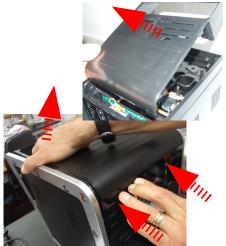
Unhook the highlighted frame and press and lift the top cover.
