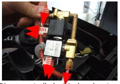
Disconnect all electrical and water circuit connections (Moltio Milk One Touch Carafe)
