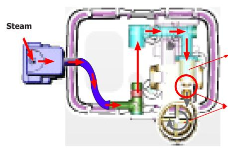
The steam passes through the pipe creating a sucking effect that pulls the milk upwards
