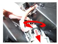
Unscrew the pump from the safety valve and slip off the pump off the upper support
