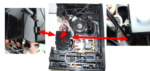
Remove the cover of the boiler by pressing the two sides with the help of a screwdriver
