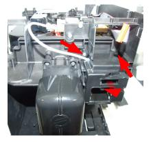
Loosen the screws and remove the assembly graft milk carafe (Moltio One Touch Milk Carafe)
