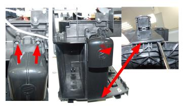
Loosen the screws and remove the assembly dispenser coffee proceeding as in the picture
