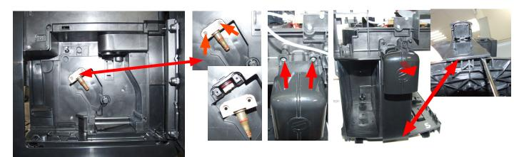
Loosen the screws as illustrated and remove the boiler pin
