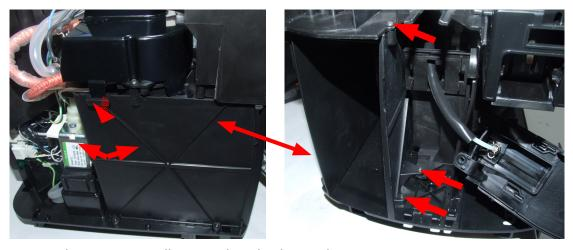
Loosen the screws as illustrated and release the insert in the bottom of the body to obtain easy access for valve disassembly
