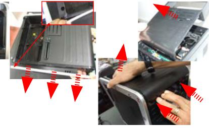
Unhook the highlighted frame and press and lift the top cover.
