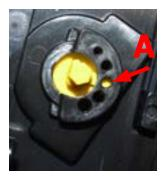
To adjust grinding further, the tecnical service can work directly on the coffee grinder by pressing and turning the ring nut (C) shown. (clockwise + to increase the particle size of the coffee and anticlockwise - to decrease it).
