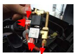
Disconnect all electrical and water circuit connections (Moltio Milk One Touch Carafe)
