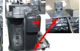
Loosen the screws as illustrated and remove the boiler pin
