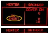
**ERROR**: In the indication **HEATER** appears **"SHORT"**, the NTC temperature-sensor is shorted, the display backlight changes from green to red; check the wiring from the NTC temperature-sensor to the CPU/POWER board (JP13).
