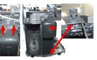
Loosen the screws and remove the assembly dispenser coffee proceeding as in the picture
