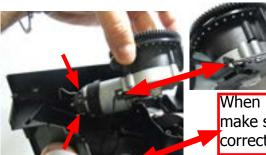
When reassembling the coffee grinder, make sure the spring is repositioned correctly (see photo).
