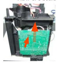
Loosen the screws slide the card off the support and disconnect the electrical connections.
