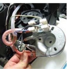
Unscrew the screw shown and remove the electrical and water circuit connections.
