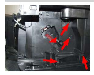
Loosen the screws as illustrated and remove the gear motor cover.
