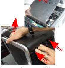
Unhook the highlighted frame and press and lift the top cover.
