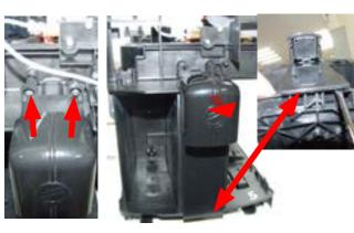
Loosen the screws and remove the assembly dispenser coffee proceeding as in the picture
