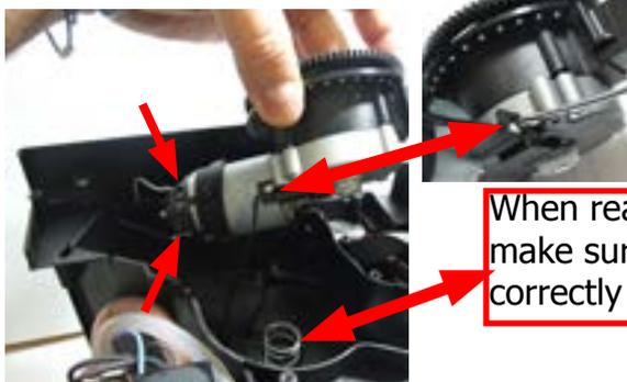
When reassembling the coffee grinder, make sure the spring is repositioned correctly (see photo).
