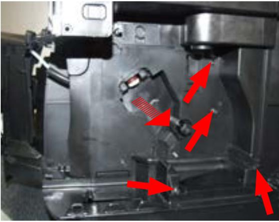
Loosen the screws as illustrated and remove the gear motor cover.
