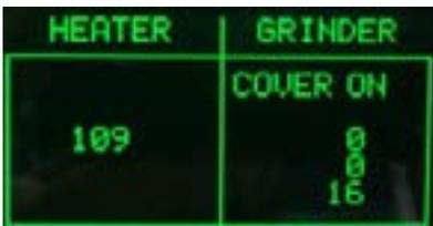
**ERROR:** if the text shown "COVER ON" / "COVER OFF" does not reflect the PRESENT / NOT PRESENT status of the Bean Hopper Cover, check the magnet presence on the cover, the REED sensor on the Bean Hopper and the REED cable to the JP25 connector onto the CPU/POWER board.
