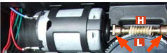
When replacing the motor and the transmission shaft, make sure the guide runners (L) are in the right position. Grease the shaft thoroughly and evenly.
