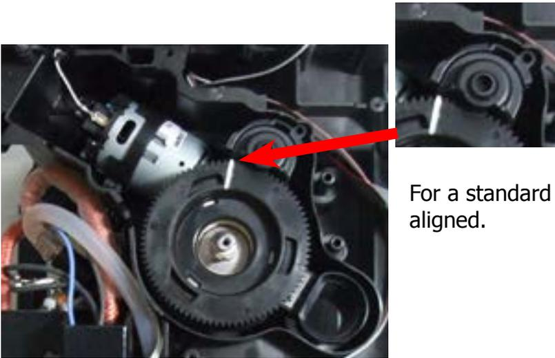
For a standard adjustment, both markings must be aligned.
