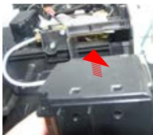
Remove the cover, loosen the screws and support teflon tube
