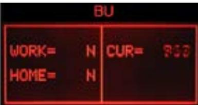
**ERROR: (Without BU)** The absorbed current is higher than 200mA, the display backlight changes from green to red; check the BU and the motor.
