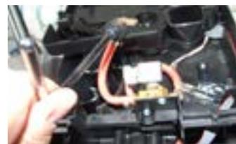
Disconnect the water circuit connection
