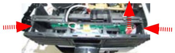
Disconnect the electrical connections. Press to right and left and lift the assembly KYB.
