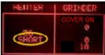
**ERROR:** In the indication HEATER appears "SHORT", the NTC temperature-sensor is shorted, the display backlight changes from green to red; check the wiring from the NTC temperature-sensor to the CPU/POWER board (JP13).
