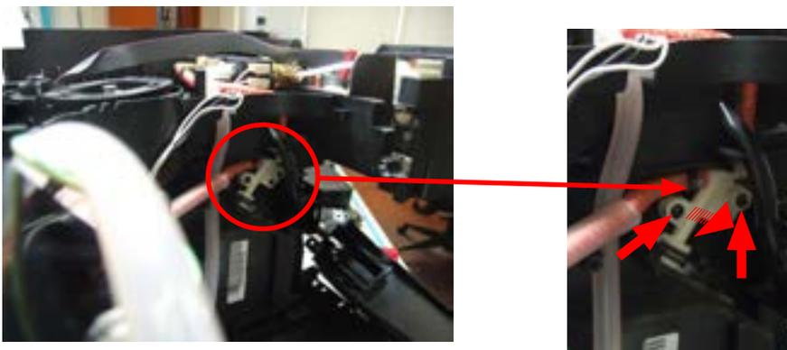
Loosen the screws as illustrated, remove the hydraulic connections and take out the valve
