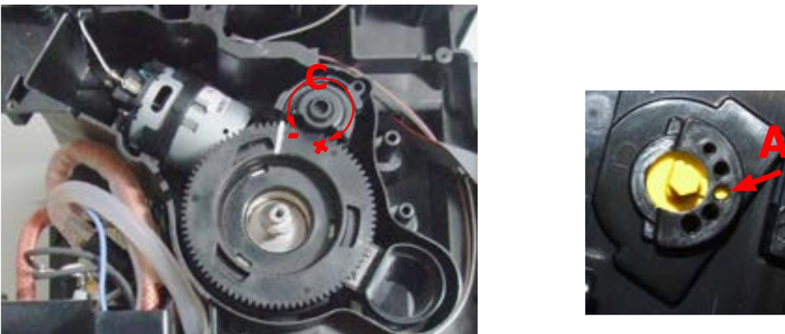
To adjust grinding further, the technical service can work directly on the coffee grinder by pressing and turning the ring nut (C) shown. (clockwise + to increase the particle size of the coffee and anticlockwise - to decrease it).
