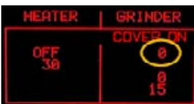
**ERROR:** The number remains 0 or the grinder does not run, the display backlight changes from green to red; check the Hall sensor board of the Grinder, the Grinder, the wiring from the Hall sensor board to the CPU/POWER board (JP2) and the wiring from the Grinder to the CPU/POWER board (JP8)
