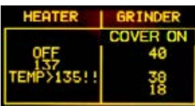
If temperature is over 135°C, the backlight change from GREEN to YELLOW. This is a ALERT message to avoid heating the HEATER element over dangerous temperature.
