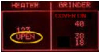
**ERROR:** In the indication HEATER appears "OPEN", the NTC temperature-sensor is detached or broken, the display backlight changes from green to red; check the wiring from the NTC temperature-sensor to the CPU/POWER board (JP13).
