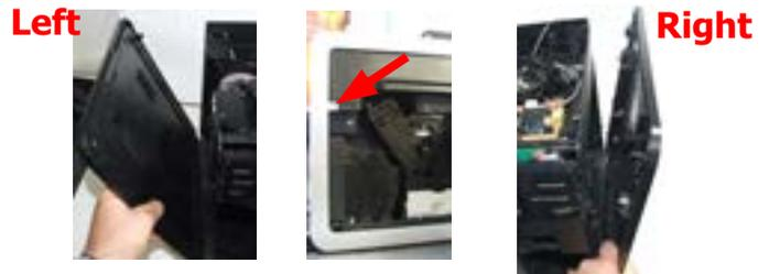
Unscrew the screw shown and remove the lateral panels
