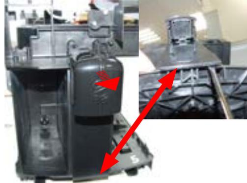
Loosen the screws and remove the assembly graft milk carafe (Moltio One Touch Milk Carafe)
