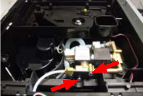
Loosen the screws holding the solenoid valve to the upper plate
