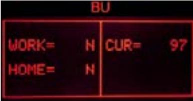
**ERROR:** The indication **HOME** doesn't change and remain "N", the display backlight changes from green to red; Check the work microswitch (is broken), the BU motor (is blocked) and the wiring (JP16).
