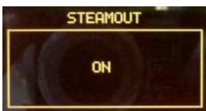
When the machine is switched on the procedure starts; the display changes to yellow and the word "ON" indicates that the procedure is running. During the procedure the 2-way solenoid valve remains open and the steam is discharged.
