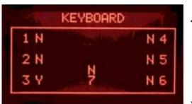
The letter next to it changes from N to Y when only one button is pressed. By pressing buttons 1, 3, 4, 6 the display color changes from GREEN to RED. By pressing buttons 2, 5 and 7 the display color changes from GREEN to YELLOW.
