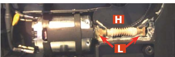
When replacing the motor and the transmission shaft, make sure the guide runners (L) are in the right position.
