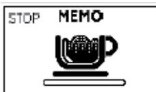
The machine is programming the amount of milk to be dispensed in order to prepare a cappuccino.
