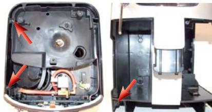
Loosen the screws as illustrated and remove the left side body.
