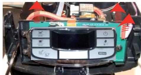
Disconnect the electrical connections and unhook the card support.
