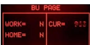
Press the espresso button to move the brewing unit to the "HOME" position
