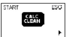
If this page is displayed after starting the machine, this means that the descaling cycle is needed. Press the "MEMO" button to enter the descaling menu and refer to the relevant section. Press the "MEMO" button to go on using the machine. Please bear in mind that failure to descale your machine will prevent it from working properly. Repair is not covered by warranty.
