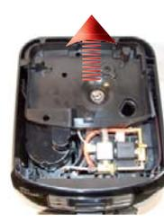
Loosen the screws as illustrated, slide out the rear body and the sound insulating cover of the coffee grinder.
