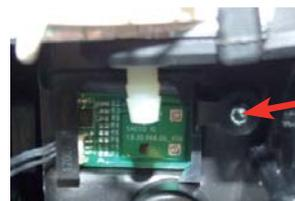
Loosen the screw as illustrated and remove the capacitive sensor glued to the seat.
