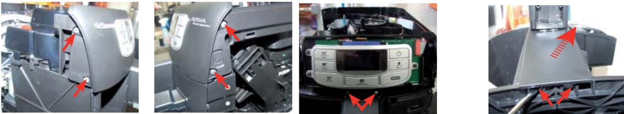
Loosen the screws highlighted and the remove the front cover panel.
