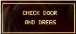
If the dreg drawer is in position and the side hatch closed, the EV cannot be done. If it is not in the right position, a warning message is shown on the display, which turns yellow.
