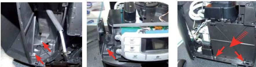
Loosen the screws as illustrated and release the insert in the bottom of the body to obtain easy access for valve disassembly
