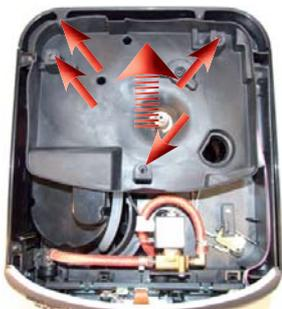
Loosen the screws as illustrated and remove the sound insulating cover. Raise the coffee grinder and remove the connections.
