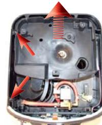
Loosen the screws as illustrated, slide out the rear body and the sound insulating cover of the coffee grinder.
