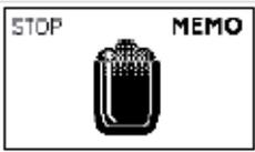
The machine is programming the amount of milk to be dispensed in order to prepare a Latte Macchiato.
