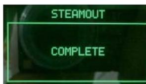
When the procedure is completed, the message "COMPLETE" appears on the display, the solenoid valves close automatically and the machine may be switched off.
