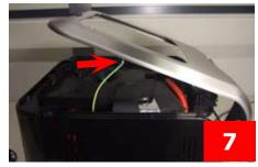
**7**) Lift the lid and disconnect the earth wire shown
