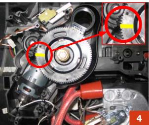
**4)** When refitting the upper grinder support, make sure you reposition it so that the mark is as illustrated in the photo
