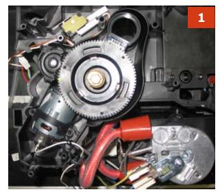
1) To remove the coffee grinder, simply slide it out and remove its connections
