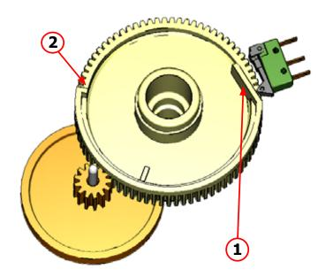
The gear motor is powered by a direct current motor that engages with the smaller double toothed wheel using a worm screw. The unit is mounted on the axle of the large gear wheel and when a coffee is requested, it moves from the home position to the dispensing position, and then back to the home position again.
