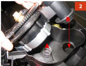
**2)** When replacing it, make sure the spring (A) and the coffee pipe (B) are positioned correctly
