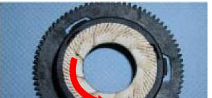
**2)** To remove the grinder blade from the upper support, turn it anti-clockwise until it detaches from the bayonet coupling
