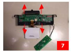
**7**) Release the keypad circuit board and disconnect the display
