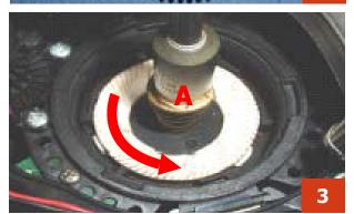
**3)** To remove the lower grinder blade, keep the increment pin (A) locked in position and turn the grinder blade anti-clockwise, until it detaches from the bayonet coupling
