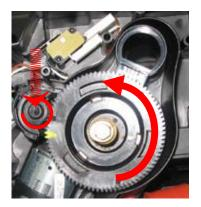
**1)** To remove the upper grinder support, using a hex key push down and turn clockwise to release the grinder support from the bayonet coupling
