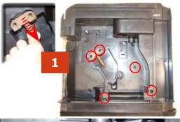
**1**) Loosen the screws holding the boiler pin in place, remove it and loosen the other screws shown
