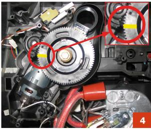
**4)** When refitting the upper grinder blade support, make sure it is placed as shown in the picture, with the highlighted mark in the same position.
