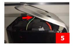
**5)** Lift the upper cover and disconnect the earth wire shown.
