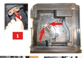
**1**) Remove the boiler pin by loosening the screws shown.
