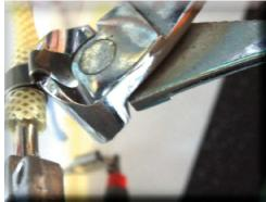
Use a suitable pair of pliers to remove the clamp (as shown).
