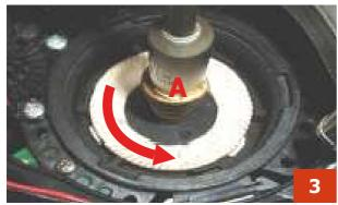
**3)** To remove the lower grinder blade, block the increment pin (A) in place and turn the grinder blade anti-clockwise until it is released from the bayonet coupling.
