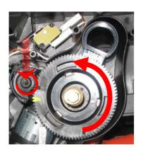
1) To remove the upper grinder blade support, use an Allen wrench and turn it clockwise to release it from the bayonet coupling.
