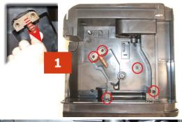
**1**) Loosen the screws of the boiler pin, remove it and loosen the others shown.
