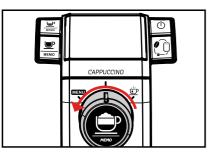
Turn the selector anti-clockwise until "MENU" is reached in order to access the programming menu in appliance ready mode
