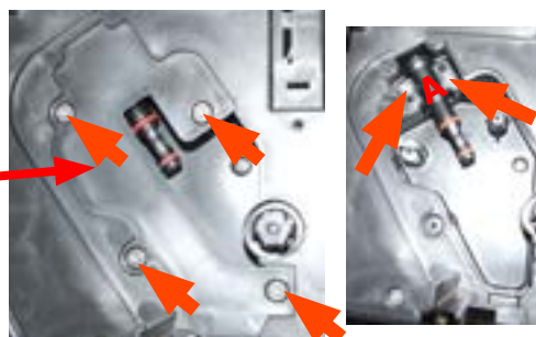
Loosen the screws as illustrated and remove the boiler pin (A).
