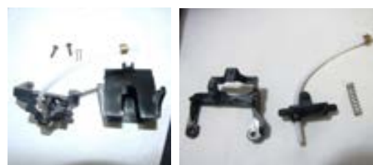
When reassembling the assembly to be careful to correctly position the spring.
