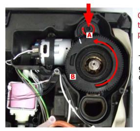
Caution in the new coffee grinder with the screw, Unscrew this last, before disassembly of the upper coffee grinder support.
