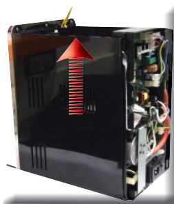
Unscrew the screws as indicated under the water container cover (A) and the coffee bean hopper (B). Unhook and gently raise the casing cover (C) by a few cm. Go onto the opposite side and raise the cover as shown in the photo (D)
