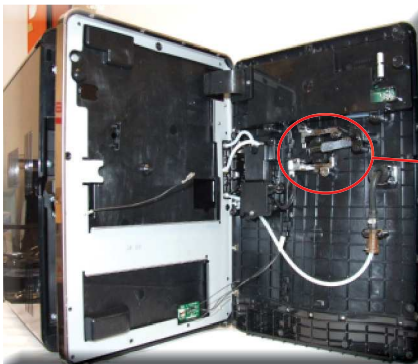
Loosen the screws located inside the door and slide out the coffee dispenser as shown
