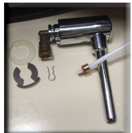
Remove the fork spring and the steam pipe washer, disconnect the pipe from the Teflon by removing the fork
