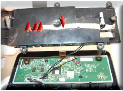
Extract the connections and flat cable.
