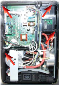
Loosen the screws as indicated and remove the rear frame
