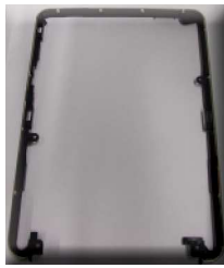
Loosen the screws as indicated and remove the rear frame
