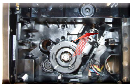
Raise the coffee grinder and remove the connections
