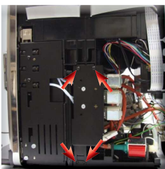
Unscrew the screws anchoring the valve support to the housing and to the horizontal plate as shown
