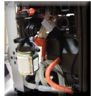
Disconnect the electrical and water circuit connections
