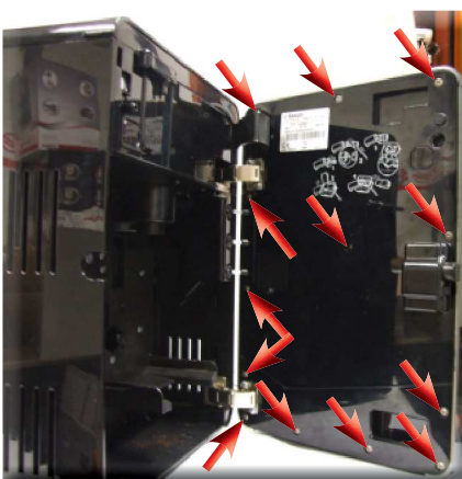
Loosen the screws as illustrated to remove the inner front panel cover
