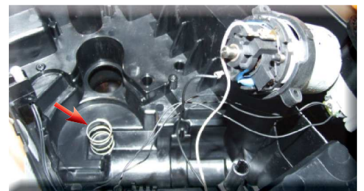
When reassembling the coffee grinder, make sure the spring is repositioned correctly (see photo)
