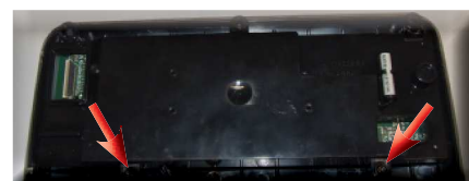
Unscrew the screws of the display support as shown
