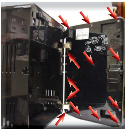
Loosen the screws as illustrated to remove the inner front panel cover
