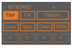
This is the button test page: each beverage corresponds to a box on the display that changes colour when the corresponding button is pressed (e.g.: ESPRESSO)
