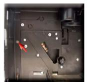
Unscrew the screws as indicated to reach the screw anchoring the multi-way valve to the support
