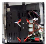
Unscrew the screws anchoring the valve support to the housing and to the horizontal plate as shown
