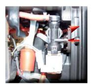
Loosen the screw as illustrated and remove the clip
