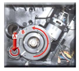
To extract the top support of the appliance, press on the grinding adjustment spindle (A) and turn the support anticlockwise until it unhooks.
