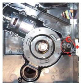
To adjust grinding further, the engineer can work directly on the coffee grinder by pressing and turning the ring nut (C) shown. (clockwise + to increase the particle size of the coffee and anticlockwise - to decrease it).
