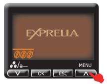
Press the "MENU" button to go to the machine's main menu
