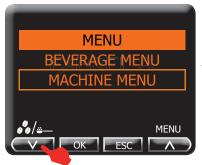
Press the "OK" button to go to the MACHINE MENU
