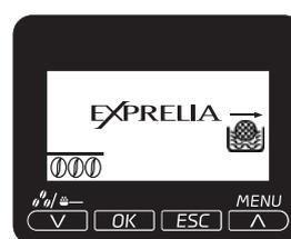
The machine requires replacement of the "Intenza" filter with a new one. The alarm is displayed only if the "enable filter" function is ON.
