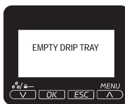
Open the front hatch and empty the drip tray underneath the brewing unit. You should also empty the dreg drawer, as the dregs counter will also be reset when the machine is switched on.
