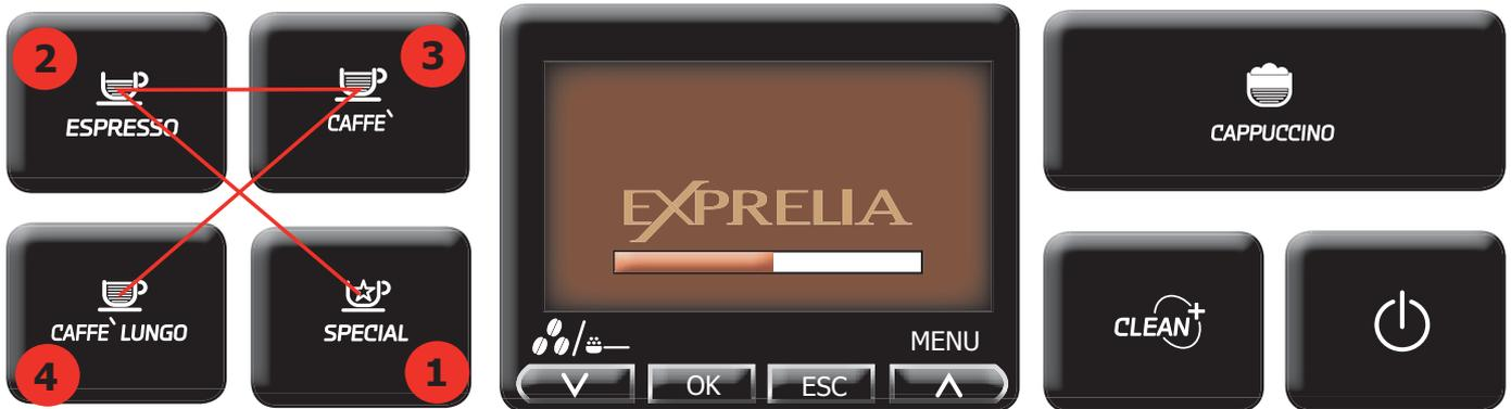
Entry into Test Mode results in a screen divided into sections, as illustrated in the diagram below
