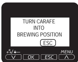
A beverage with milk has been selected. The machine requires the carafe handle spout to be placed into dispensing position. Press the button "ESC" to cancel the selection
