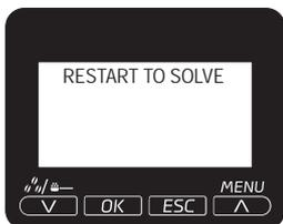
An event has occurred which requires the machine restart. Take note of the code (E xx) shown at the bottom. Switch off the machine, wait 30 seconds and then switch it on again. If the problem persists, contact the service centre.
