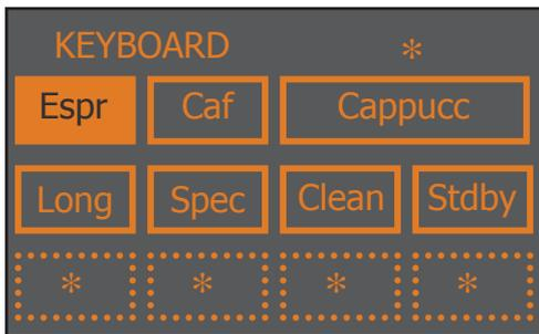
This is the button test page: each beverage corresponds to a box on the display that changes colour when the corresponding button is pressed (e.g.: ESPRESSO)
