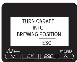
A beverage containing milk has been selected. The machine asks you to place the carafe handle spout in its dispensing position. Press "ESC" to cancel the procedure
