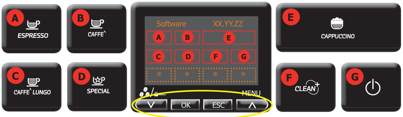
The sectors highlighted in red on the following screens represent the various loads that can be activated by pressing the corresponding keys on the keypads.
