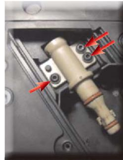
Loosen the screws as illustrated and remove the boiler pin
