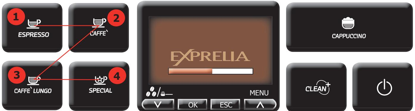
Entering Diagnosis Mode shows a screen like the one in the following diagram and pressing
