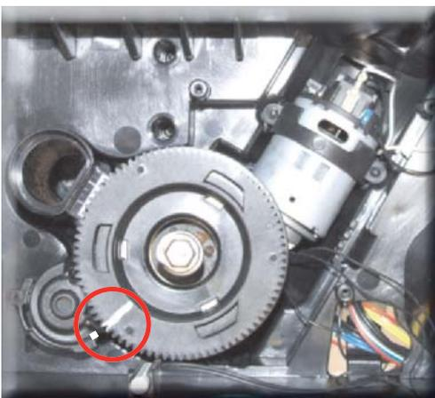
For a standard adjustment, both markings must be aligned.
