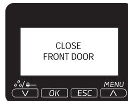
For the machine to become operative, the service hatch must be closed
