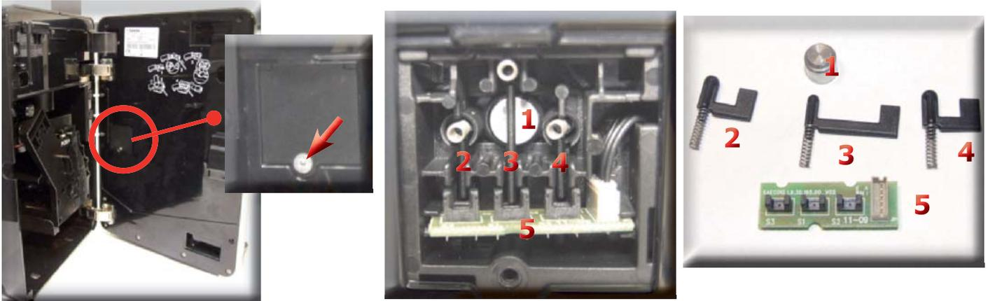
Loosen the screw as shown
