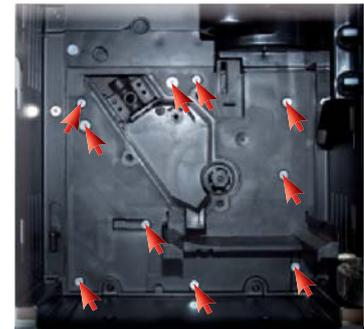
Loosen the screws as illustrated and remove the gearmotor cover
