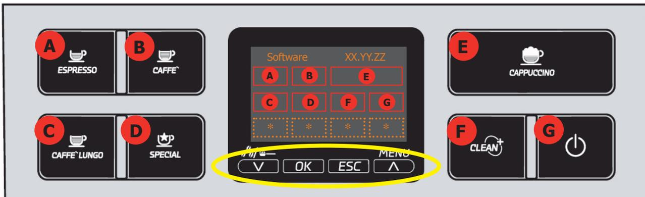
The sectors highlighted in red on the following screens represent the various loads that can be activated by pressing the corresponding keys on the keypads.
