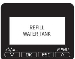
Take out the tank and fill it with fresh drinkable water or top it up by means of the special port.
