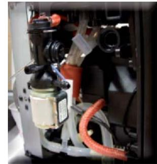
Disconnect the electrical and water circuit connections
