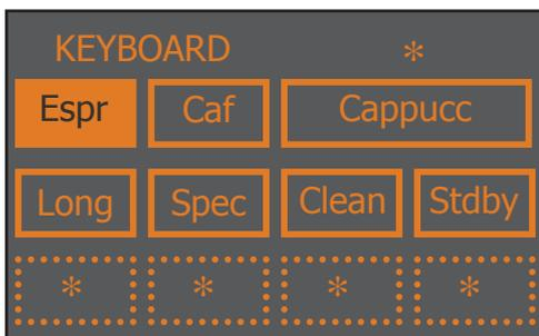
This is the button test page: each beverage corresponds to a box on the display that changes colour when the corresponding button is pressed (e.g.: ESPRESSO)
