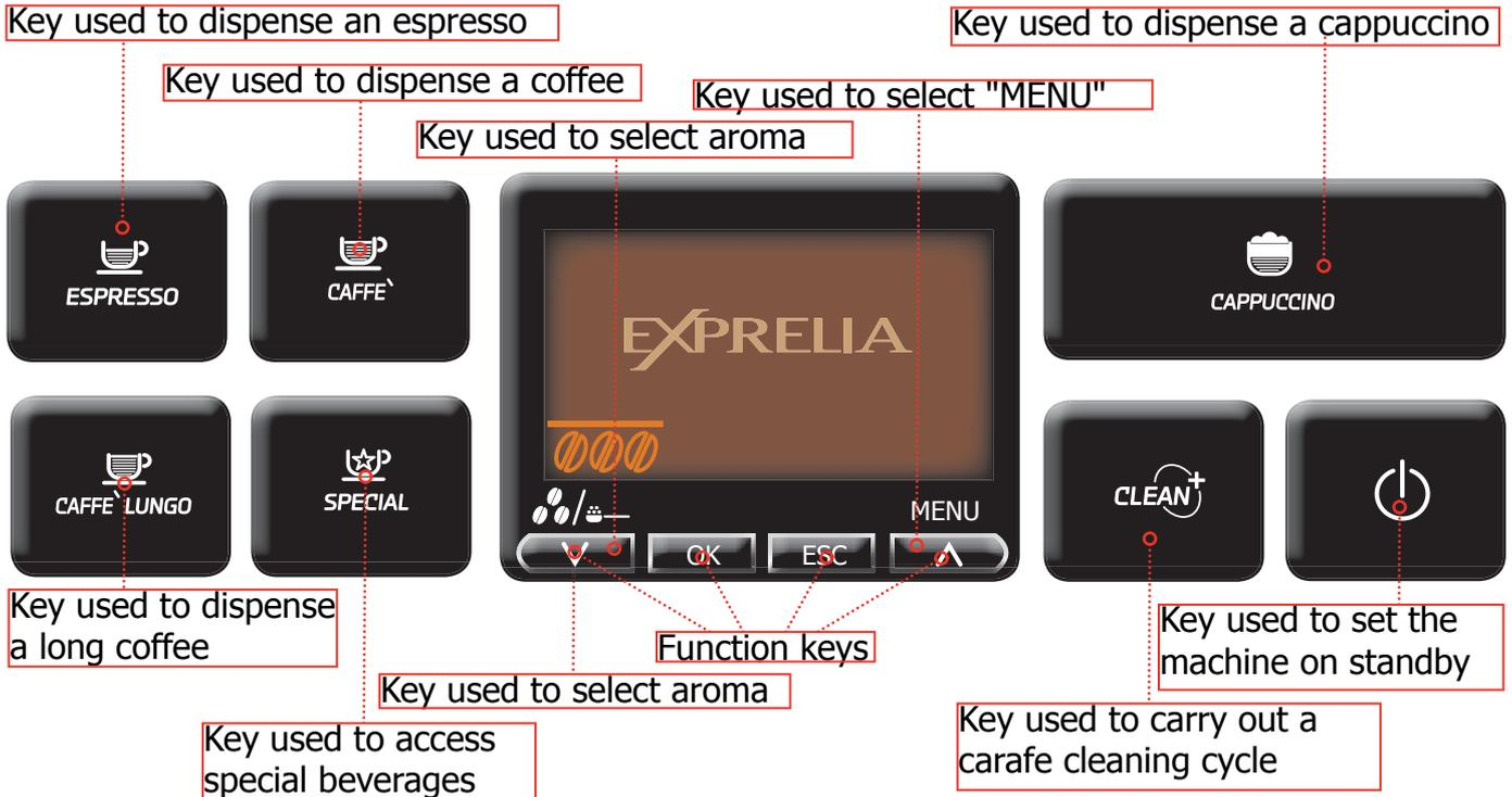
**BEVERAGE MENU** The machine allows custom settings for dispensing each beverage
