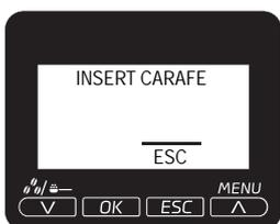
An operation has been selected that requires dispensing from the milk container. Insert the milk container. Press "ESC" to cancel the procedure
