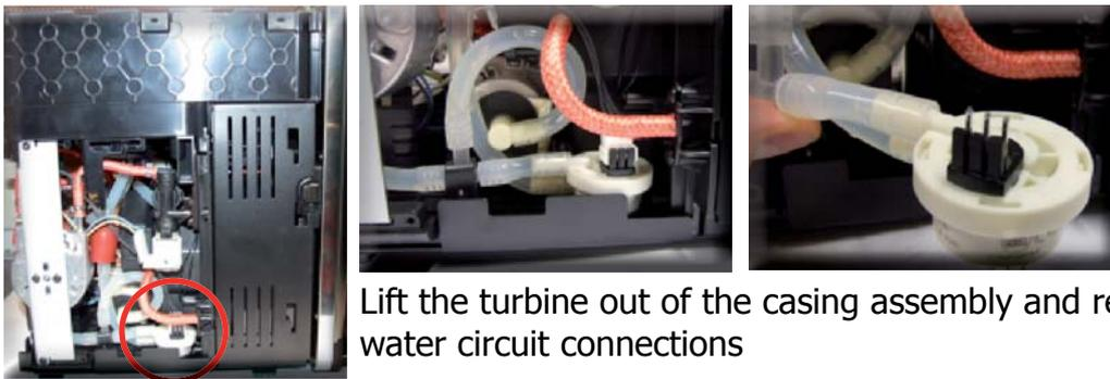
Lift the turbine out of the casing assembly and remove the electrical and water circuit connections
