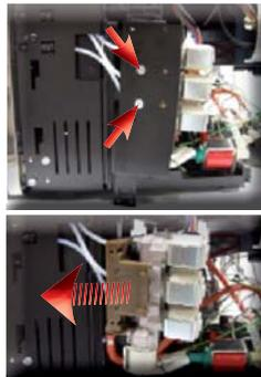
Unscrew the screws shown and pull out the valve assembly
