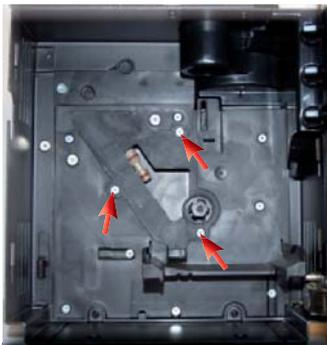
Loosen the screws as illustrated and remove the boiler pin
