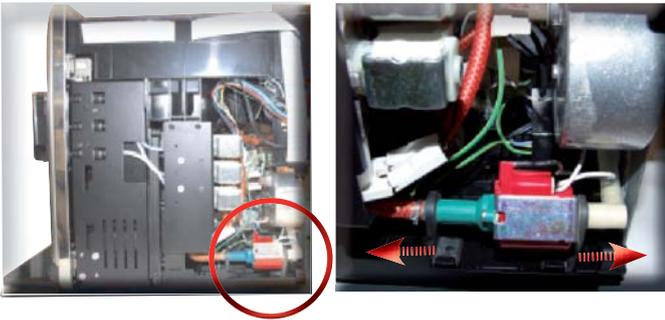
Slide out the two pump supports (highlighted) fixed to the housing and disconnect the electrical and water circuit connections
