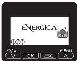
The machine requests the "Intenza" water filter to be replaced with a new one. Replace the filter as described on page 7. The alarm is displayed only if the "Enable Filter" function is set to "ON".
