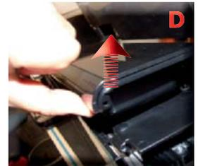
Unscrew the screws as indicated under the water container cover (A) and the coffee bean hopper (B). Unhook and gently raise the casing cover (C) by a few cm. Go onto the opposite side and raise the cover as shown in the photo (D)
