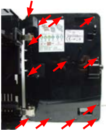
Loosen the screws as shown to remove the inner cover of the front panel
