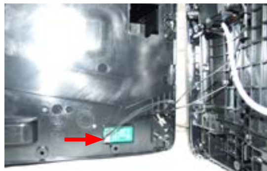
Loosen the screws as shown to remove the inner cover of the front panel and disconnect the electrical connections
