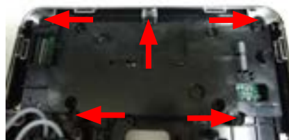
Loosen the screws as shown and remove the CPU board assembly
