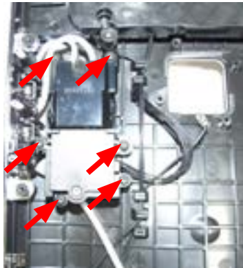
Loosen the screws as shown and the Teflon pipe support cover from the carafe
