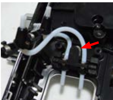
When re-mounting it, make sure to reposition the spring correctly
