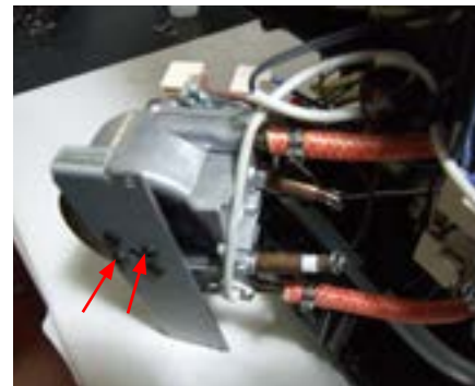
Loosen the screw as shown and remove the electrical and water connections
