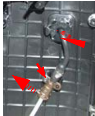
Loosen the screw and remove the steam pipe and disconnect the pipe from the Teflon by removing the fork
