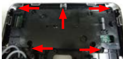
Loosen the screws as shown and remove the CPU board assembly
