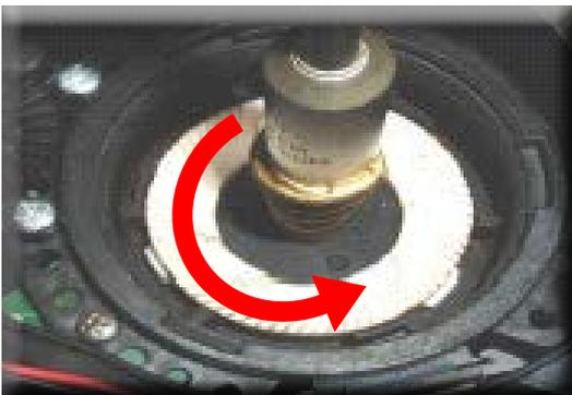
Turn the grinder blades anticlockwise out of the support.
