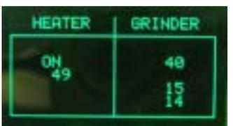
**Press the ESPRESSO button to switch on the Heater**
