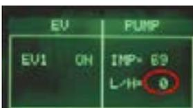
**ERROR:** The L/H is zero or very low; the Electro Valve does not open. Check the wiring from the Electro Valve to the CPU/POWER board (JP3) and the Electro Valve.
