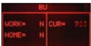
**ERROR: (Without BU)** The absorbed current is higher than 200mA, the display backlight changes from green to red; check the BU and the motor.
