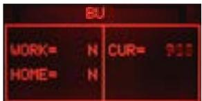
**ERROR: (Without BU)** The absorbed current is more than 200mA, the display backlight changes from green to red; check the BU and the motor.
