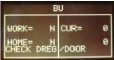
**Press the ESPRESSO button to move the BU to Work**
