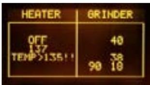
If temperature is over 135°C, the backlight change from GREEN to YELLOW. This is a ALERT message to avoid heating the HEATER element over dangerous temperature.
