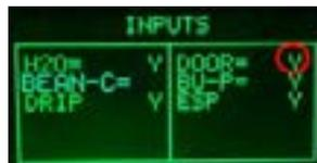
ERROR: The indication DOOR does not change; check the Microswitch for the door and the wiring (JP14). NOTE: without the Dreg Drawer correctly inserted the DOOR indication cannot change !
