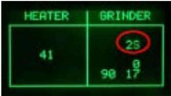
**Press the STEAM button to switch on the grinder**
