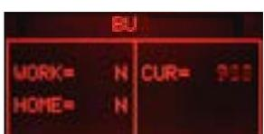
**ERROR: (With BU)** The absorbed current is higher than 300mA, the display backlight changes from green to red; check the BU and the motor
