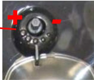
The grinding adjustment can be set by the user (only with the coffee grinder in operation) by pressing and turning (only by one click at a time) the insert inside the coffee bean hopper with the aid of the wrench supplied.
