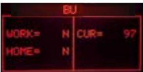
**ERROR:** The indication **WORK** doesn't change and remain "N", the display backlight changes from green to red; Check the work microswitch (broken?), the BU motor (blocked?) and the wiring (JP16)
