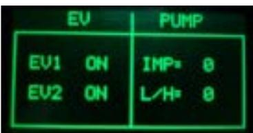
**Press the COFFEE button to open the Electro Valve 2**
