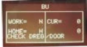
**Press the Z1 button to move the BU to Work**
