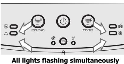
Turn off the machine. After 30 seconds, turn it on again. Repeat the procedure 2 or 3 times.
