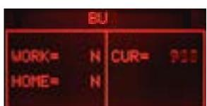
ERROR: **(With BU)** The absorbed current is higher than 300mA, the display backlight changes from green to red; check the BU and the motor
