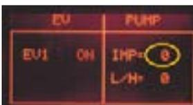
**ERROR:** The display backlight changes from green to red and the impulse remains 0; If water comes out the pipe: check the wiring from the flowmeter to the CPU/POWER board (JP5). If no water comes out the pipe: check the pump and the wiring from the pump to the CPU/POWER board (JP24).
