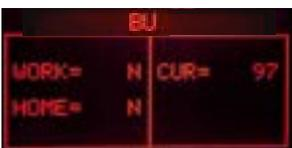
**ERROR:** The indication **HOME** doesn't change and remain "N", the display backlight changes from green to red; Check the work microswitch (is broken), the BU motor (is blocked) and the wiring (JP16).
