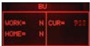
ERROR: **(Without BU)** The absorbed current is more than 200mA, the display backlight changes from green to red; check the BU and the motor.
