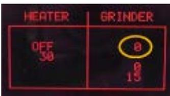
**ERROR:** The number remains 0 or the grinder does not run, the display backlight changes from green to red; check the Hall sensor board of the Grinder, the Grinder, the wiring from the Hall sensor board to the CPU/POWER board (JP2) and the wiring from the Grinder to the CPU/POWER board (JP8)
