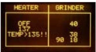
If temperature is over 100°C, the backlight change from GREEN to YELLOW. This is a ALERT message to avoid heating the HEATER element over dangerous temperature.
