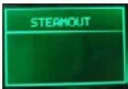
Once entered the Steam Out mode the display shows the "STEAM OUT" indication. Buttons can be released
