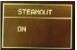
The machine starts the Steam Out and the display change the backlight (yellow) and appears the indication "ON". While the Steam Out runs the Electrovalve is opened and water comes out the Water/Steam pipe.
