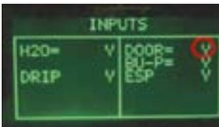
ERROR: The indication DOOR does not change; check the Microswitch for the door and the wiring (JP14). NOTE: without the Dreg Drawer correctly inserted the DOOR indication cannot change !
