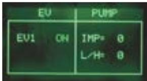
It is possible to hear the "click" from Electro Valve. The indication beside the **EV1** changes from "OFF" to "ON".
