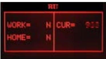
**ERROR:** (Without BU) The absorbed current is more than 200mA, the display backlight changes from green to red; check the BU and the motor.
