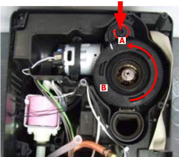
To extract the top support of the appliance, press on the grinding adjustment spindle (A) and turn the support anticlockwise until it unhooks.
