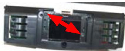
Loosen the screws for remove the cover.
