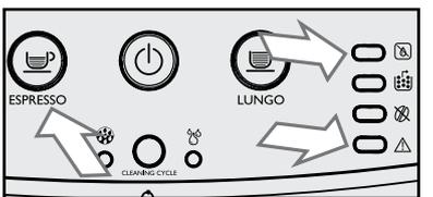
You have to prime the machine by pressing the espresso button. Once pressed, the "☕" button turns off. During priming the "⊠" and "⚠" keep on flashing. They stop flashing when the priming is finished.
