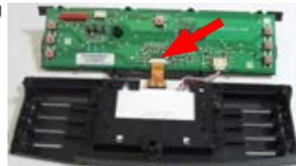
Disconnect the electrical connections.
