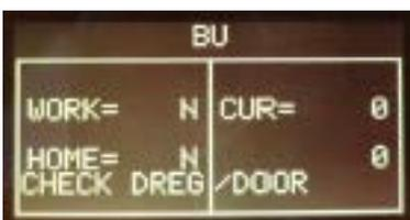
**Press the ESPRESSO button to move the BU to Work**
