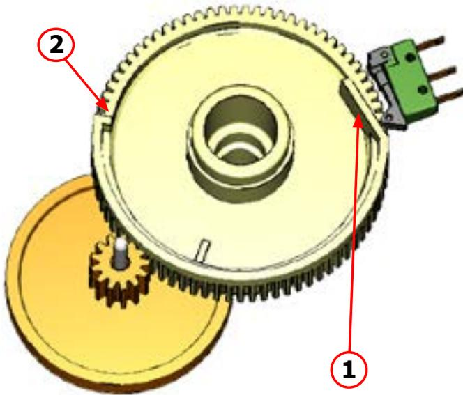
The gear motor is powered by a direct current motor that engages with the smaller double toothed wheel using a worm screw. The unit is mounted on the axle of the large gear wheel and when a coffee is requested, it moves from the standby position to the dispensing position, and then back to the standby position again.
