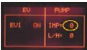
**ERROR:** The display backlight changes from green to red and the impulse remains 0; If water comes out the pipe: check the wiring from the flowmeter to the CPU/POWER board (JP5). If no water comes out the pipe: check the pump and the wiring from the pump to the CPU/POWER board (JP24).
