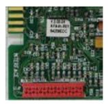
The firmware version is the same as the label on MicroController
