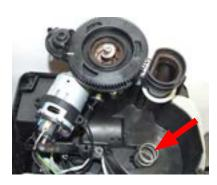
When reassembling the coffee grinder, make sure the spring is repositioned correctly (see photo).
