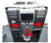
Unscrew the screw shown Press the sides and remove the cover and dispenser. Insert as before to reassemble the dispenser in the rail and then the coverage.
