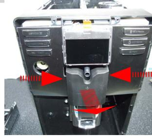
Press the sides and remove the cover and dispenser. Insert as before to reassemble the dispenser in the rail and then the coverage.
