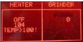
If temperature is over 100°C, the backlight change from WHITE to RED. This is a ALERT message to avoid heating the HEATER element over dangerous temperature.
