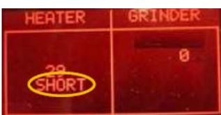
**ERROR:** In the indication **HEATER** appears "**SHORT**", the **NTC** temperature-sensor is shorted, the display backlight changes from white to red; check the wiring from the NTC temperature-sensor to the CPU/POWER board (JP13).
