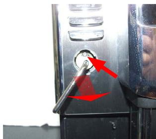
Remove the cap, unscrew the screw shown and remove the steam tube.
