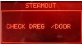
**IMPORTANT NOTE:** to execute the Steam-Out procedure the DREGDRAWER must be in place and the DOOR must be closed. If these 2 conditions are not respected a warning message is shown on the display and the Steam-Out is interrupted.
