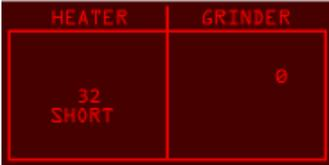
ERROR: In the indication HEATER appears "SHORT", the NTC temperature-sensor is shorted, the display backlight changes from white to red; check the wiring from the NTC temperature-sensor to the CPU/POWER board (JP13).
