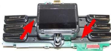
Loosen the screws for remove the cover.
