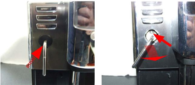
Remove the cap, unscrew the screw shown and remove the steam tube.
