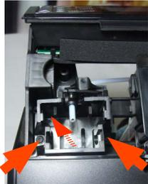
Loosen the screws holding the carafe connection
