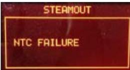
**IMPORTANT NOTE:** to execute the Steam-out procedure the Ntc sensor must work correctly; if some errors occurs on Ntc during the steam-out, the procedure can't continue and an error message is shown on the display.
