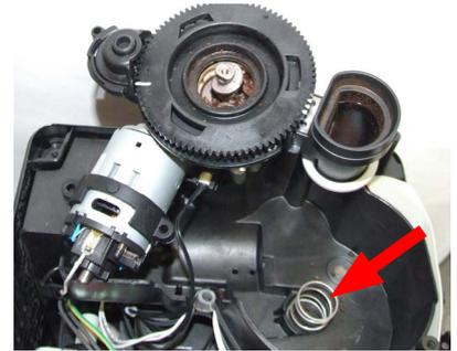
Raise the coffee grinder and remove the connections.
