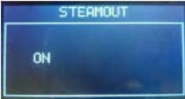
Once entered the Steam Out mode the display shows the **"STEAM OUT"** indication. Buttons can be released.
