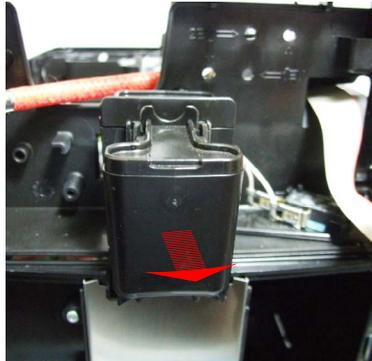
Unscrew the screws shown and remove the dispenser
