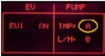
**ERROR:** The display backlight changes from white to red and the impulse remains 0; If water comes out the pipe: check the wiring from the flowmeter to the CPU/POWER board (JP5). If no water comes out the pipe: check the pump and the wiring from the pump to the CPU/POWER board (JP24).
