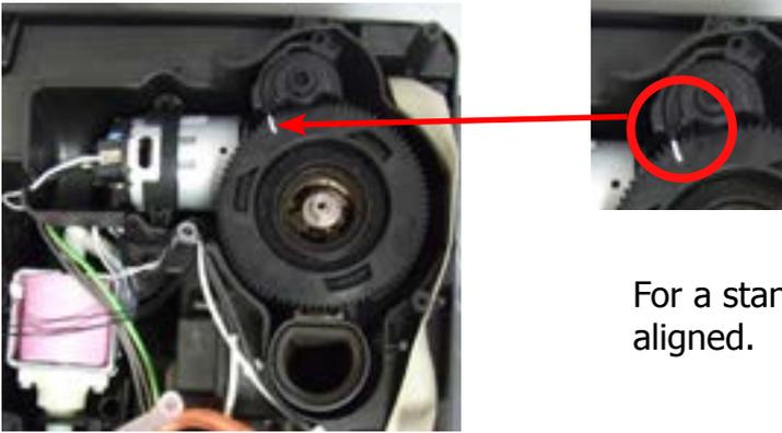
For a standard adjustment, both markings must be aligned.
