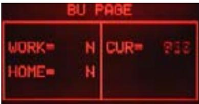
**ERROR: (With BU)** The absorbed current is more than 300mA, the display backlight changes from white to red; check the BU and the motor
