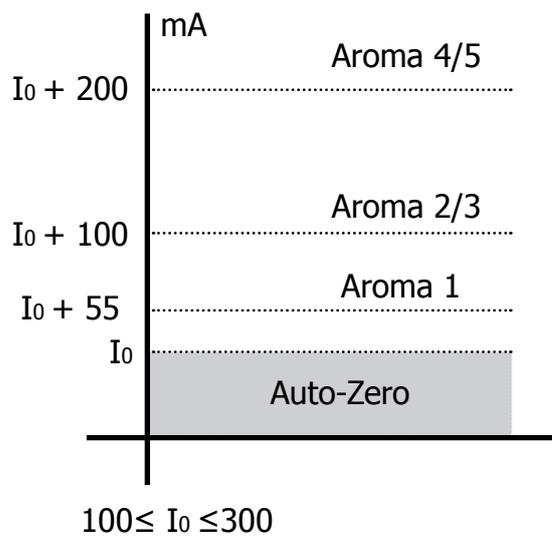
$I_0$  = current when the BU is moving without load, i.e. without coffee. It occurs, for example, during the rinsing phase of coffee spout.
