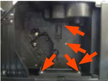
Loosen the screws as illustrated and remove the gear motor cover.
