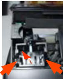
Loosen the screws holding the carafe connection
