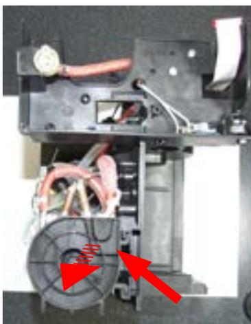
Unscrew the screw shown at unthread the support boiler
