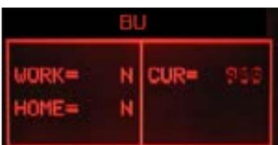
**ERROR: (Without BU)** The absorbed current is more than 200mA, the display backlight changes from white to red; check the BU and the motor.
