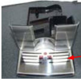
Remove the water tank, coffee container cover, drip tray, dreg drawer, brewing unit.
