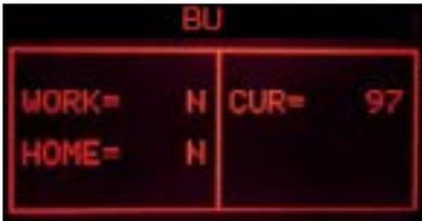
**ERROR:** The indication **HOME** doesn't change and remain "N", the display backlight changes from white to red; Check the work microswitch (is broken), the BU motor (is blocked) and the wiring (JP16)
