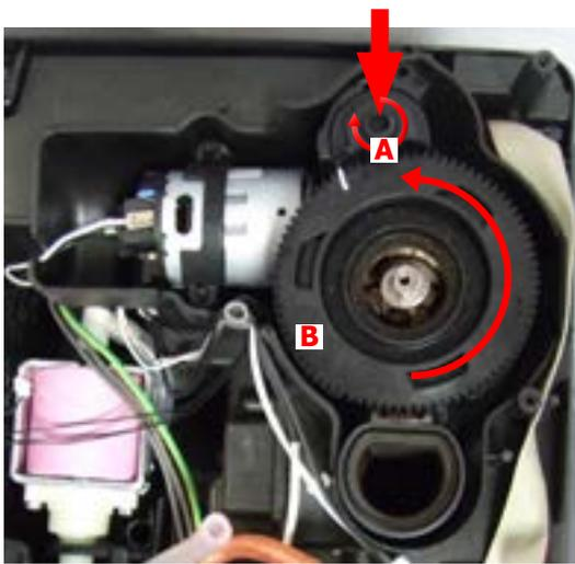
To extract the top support of the appliance, press on the grinding adjustment spindle (A) and turn the support anticlockwise until it unhooks.
