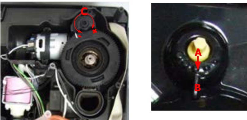
To adjust grinding further, the engineer can work directly on the coffee grinder by pressing and turning the ring nut (C) shown. (clockwise + to increase the particle size of the coffee and anticlockwise - to decrease it).
