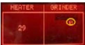
**ERROR:** The number remains 0 or the grinder does not run, the display backlight changes from white to red; check the Grinder and the wiring from the Grinder to the CPU/POWER board (JP8)
