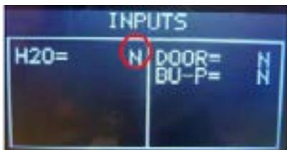
**ERROR:** The indication TANK-H2O doesn't change; check the capacitive sensor (fixing) and the wiring (JP23)
