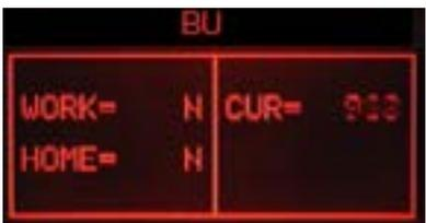
**ERROR: (With BU)** The absorbed current is higher than 300mA, the display backlight changes from white to red; check the BU and the motor.
