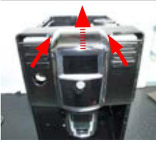
Unscrew the screw shown and remove the cover.
