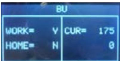
When the BU reaches the work position the indication **WORK** changes from "N" to "Y", the number of the current is less than 200mA (without BU) or 300mA (with BU).
