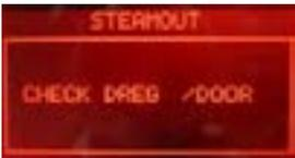
**IMPORTANT NOTE:** to execute the Steam-Out procedure the DREGDRAWER must be in place and the DOOR must be closed. If these 2 conditions are not respected a warning message is shown on the display and the Steam-Out is interrupted.
