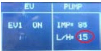
**ERROR:** The L/H is zero or very low; the Electro Valve does not open. Check the wiring from the Electro Valve to the CPU/POWER board (JP3) and the Electro Valve.
