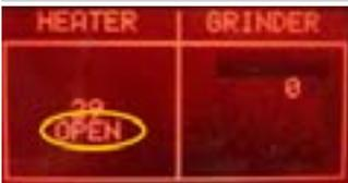
**ERROR:** In the indication **HEATER** appears “**OPEN**”, the **NTC** temperature-sensor is detached or broken, the display backlight changes from white to red; check the wiring from the NTC temperature-sensor to the CPU/POWER board (JP13).
