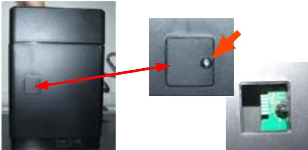
Loosen the screw for remove the cover.
