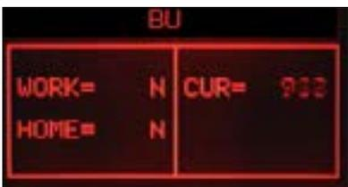
**ERROR: (Without BU)** The absorbed current is higher than 200mA, the display backlight changes from white to red; check the BU and the motor.
