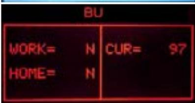
**ERROR:** The indication **WORK** doesn't change and remain "N", the display backlight changes from white to red; Check the work microswitch (broken?), the BU motor (blocked?) and the wiring (JP16).
