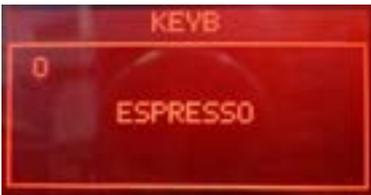
In the middle of display appears the name of the button pressed and the backlight color changes from WHITE to RED.
