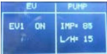
**Press and Release the Z4 button to switch on the pump (100 impulses)**
