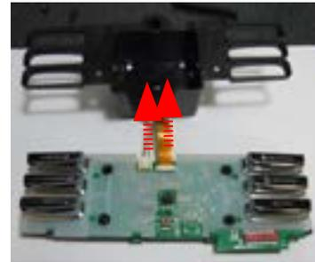
Disconnect the electrical connections.
