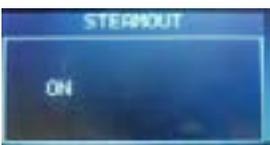
The machine starts the Steam Out and in the display appears the indication "ON".
