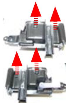
unlock where highlighted and remove the cover in the dispenser
