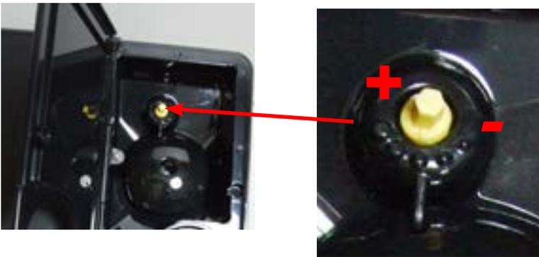
The grinding adjustment can be set by the user (only with the coffee grinder in operation) by pressing and turning (only by one click at a time) the insert inside the coffee bean hopper with the aid of the wrench supplied.
