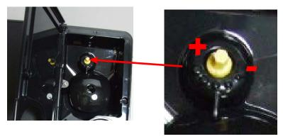
The grinding adjustment can be set by the user (only with the coffee grinder in operation) by pressing and turning (only by one click at a time) the insert inside the coffee bean hopper with the aid of the wrench supplied.
