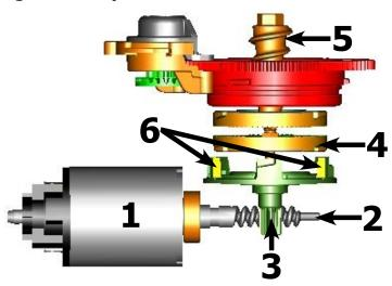
The coffee grinder is activated by a direct current motor (1) via helicoidal wheel transmission and a worm screw (2).
