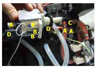
Disconnect the water circuit connections (A) and electrical connections (B), loosen the safety valve (C) and slide the pump off the brackets (D).
