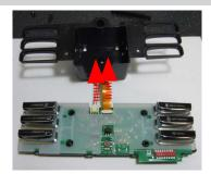
Disconnect the electrical connections.
