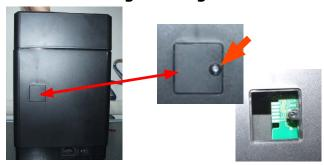
Loosen the screw for remove the cover.
