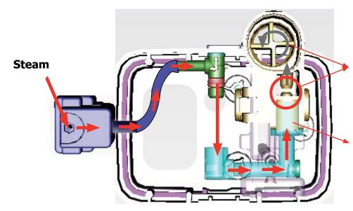
The milk is heated by the steam and taken towards the emulsion chamber where it is mixed with air and transformed into foam
