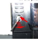
Remuve the cap, unscrew the screw shown and remove the steam tube.
