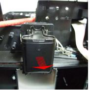
unlock where highlighted and remove the cover in the dispenser
