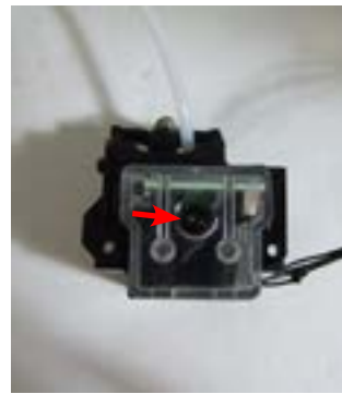
Unscrew the screws highlighted. When reassembling the assembly to be careful to correctly position the spring.
