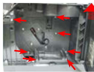
Unscrew the screws highlighted and remove the insert panel, coffee dispenser, right door and the central plate.
