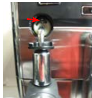
Unscrew the screws highlighted and remove the steam tube.
