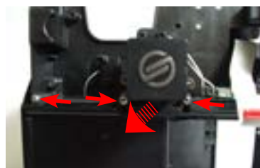
Unscrew the screws highlighted and remove the insert panel, coffee dispenser, right door and the central plate.
