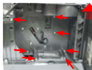
Unscrew the screws highlighted and remove the insert panel, coffee dispenser, right door and the central plate.
