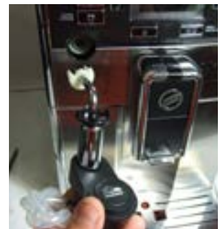
Unscrew the screws highlighted and remove the steam tube.
