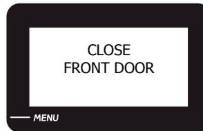
The front door must be closed for the machine to be functional
