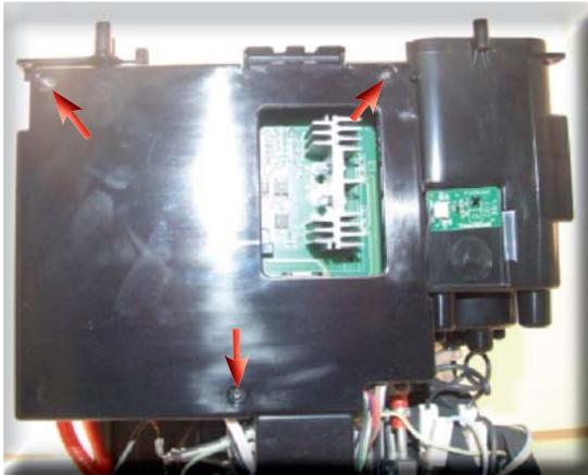
1) Loosen the screws as illustrated and remove the card cover.
