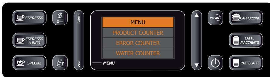
The entry to Diagnostics Mode shows a screen as seen in the figure at the side and pressing [IMG] allows to scroll through all menus present.
