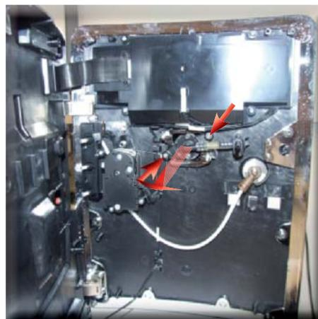
Loosen the screws as illustrated and slide out the coffee dispenser assembly (photo A).
