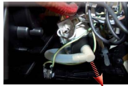
Slide out the two pump supports (highlighted) fixed to the component mounting support and disconnect the electrical and water circuit connections.
