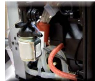
Disconnect the electrical and water circuit connections
