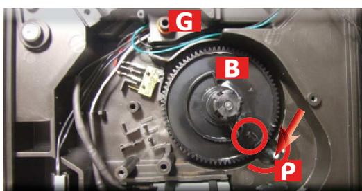
Replace the gear (B), making sure that the imprint of the arrow is aligned with the opening containing the pin (P).
