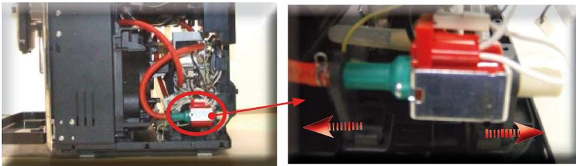
Slide out the two pump supports (highlighted) fixed to the housing and disconnect the electrical and water circuit connections.
