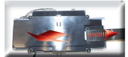
Slide out the front panel and remove the card cover, making sure you disconnect the flat cable connected to the POWER.
