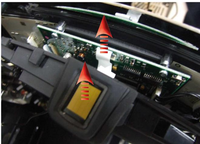
Remove the connection on the board and lift out the digital ID
