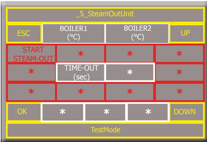
This screen corresponds to the steam\_out cycle, used to empty the coffee boiler and the hot water/steam boiler.
