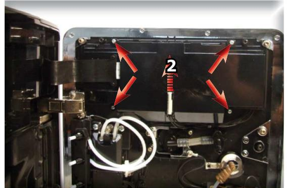
Slide the capacitive sensor out (1) along with the door presence reed sensor (2), loosen the screws highlighted and remove the CPU board cover.
