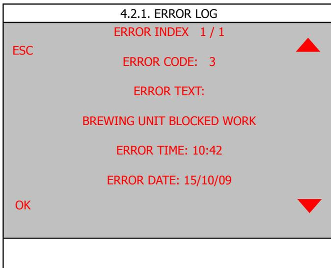
**ERROR INDEX:** displays the numerical position of the error.
