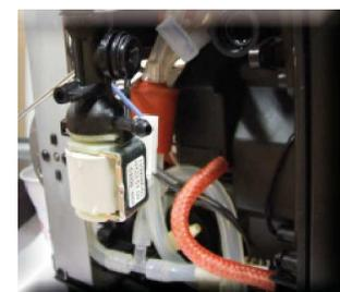
Disconnect the electrical and water circuit connections
