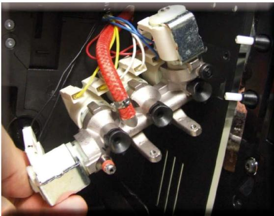
Disconnect all electrical and water circuit connections.
