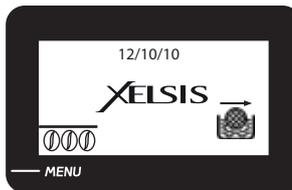
The machine notifies that the „Intenza” water filter must be replaced. The alarm is only displayed if the "Enable Filter" function is ON.
