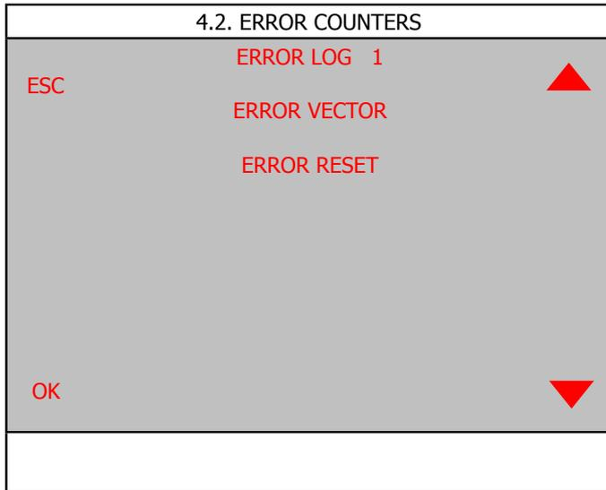
**ERROR LOG:** displays the total number of errors which have occurred in the system.
