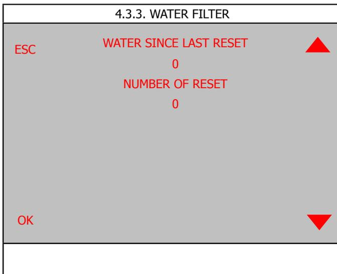
**WATER SINCE LAST RESET:** consumption of water in litres since the last time the water filter was activated (after each water filter activation procedure, the value is reset to "0").
