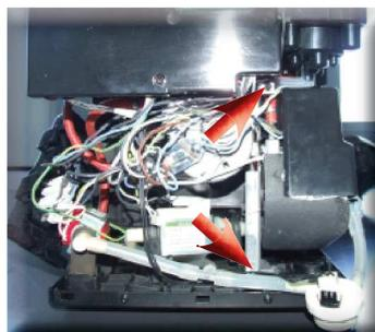
Loosen the screw as illustrated and remove the boiler cover and disconnect the electrical and water circuit connections.
