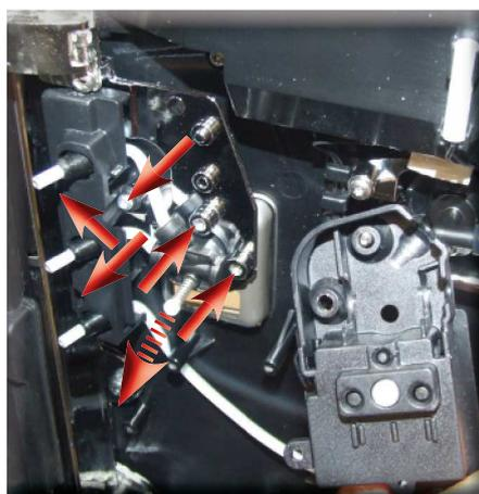
Loosen the screws as shown and slide out the spring and insert, which gives the connector its flexibility.
