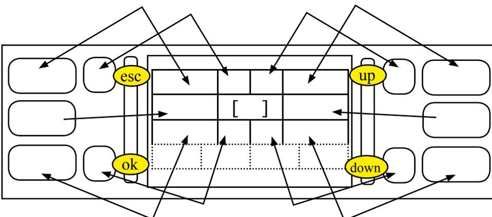
The 4 buttons (ESC, OK, UP and DOWN) highlighted in yellow, at the side of the display, can be used to scroll through the Test Mode:
