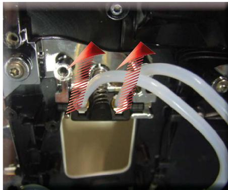
Remove the Teflon pipe support assembly
