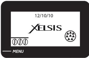
The machine requests a descaling cycle . The machine can be used with this message present but good functioning may be compromised.
