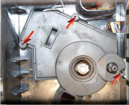
Loosen the screws as illustrated and remove the sound insulating cover of the coffee grinder.
