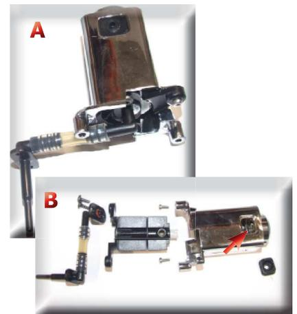
Remove the dispenser (photo B); when replacing it, make sure the spring highlighted is positioned correctly.
