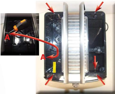
Loosen the screws as illustrated and press inside the gap (A) using a flat head screwdriver.
