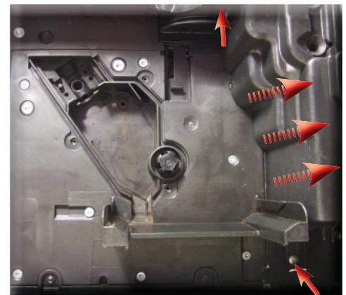
Loosen the screws as illustrated and remove the frothing valve protection.
