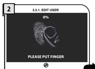
The machine will ask you to place your finger on the sensor for an initial reading
