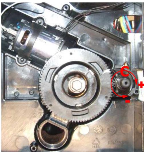
If you find ground coffee residue between the two grinders, we recommend tightening the adjustment, a max. of two notches at a time.
