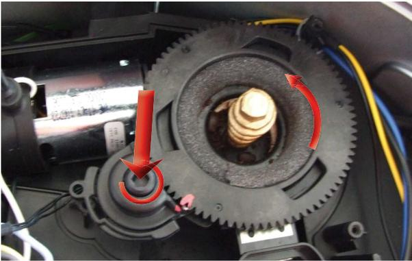
Press down on the grinder adjuster and then turn the upper grinder blades support anticlockwise until it stops.
