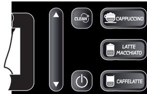
Flashing red LED. Machine in Stand-By "⏻"
