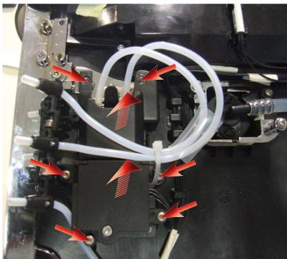
Remove the screws shown and pull out the front panel insert
