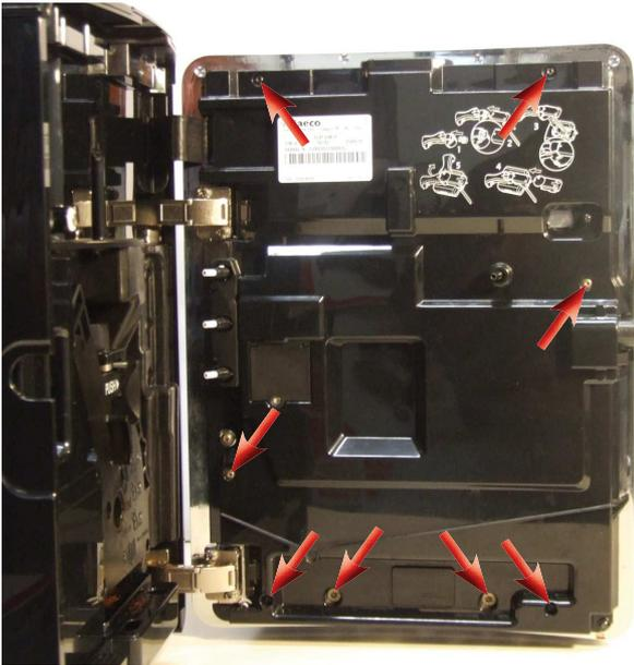
Loosen the screws as shown to remove the inner cover of the front panel
