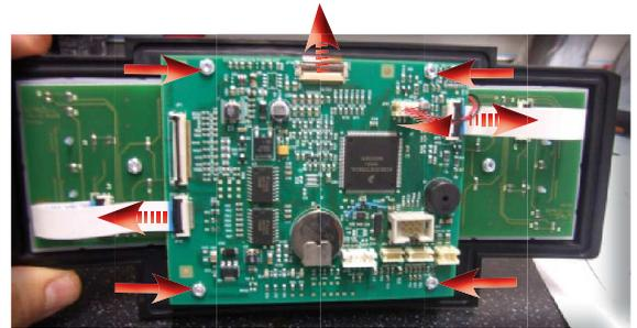
Remove the connections, loosen the screws highlighted and remove the board
