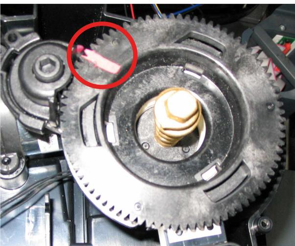
In the start position, both markings must be aligned.
