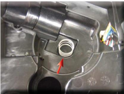
When reassembling the coffee grinder, make sure the spring is repositioned correctly (see photo).
