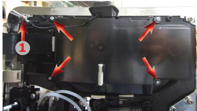
Loosen the screws as illustrated to remove the inner front panel cover.
