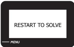
An event has occurred that requires machine re-start. Make note of the code (Exx) shown at the bottom. (see table 5.2 chap. 05 Troubleshooting) Switch the machine off and back on again after 30 seconds. If the problem repeats, contact the service centre.
