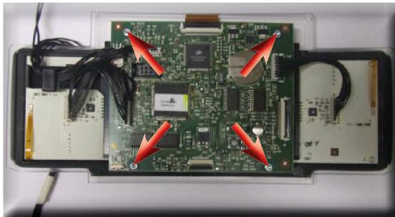
Loosen the screws as illustrated and remove all electrical connections.
