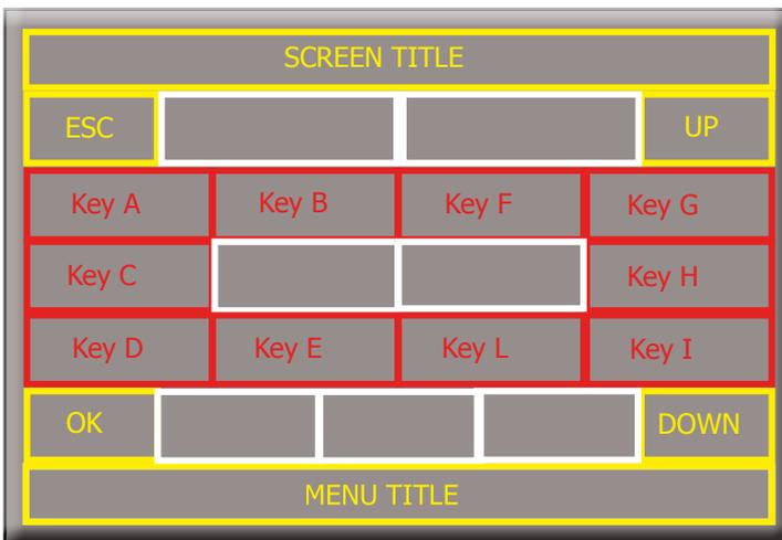
In Test Mode, all loads are initially deactivated. To activate a load, simply press the corresponding key on the keyboards at the side just once. The load is deactivated by pressing the same lined key just once. A load may be deactivated automatically when:
