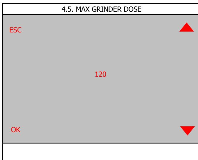
**MAX GRINDER DOSE** (can be used to select the maximum threshold value for the coffee grinder dose. The range may be set between 100 and 170, with intervals of 5).
