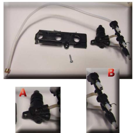
Loosen the screws as illustrated to remove the cafare attachment (A) and the Teflon pipe support (B).
