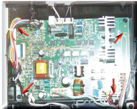
2) Loosen the screws as illustrated and remove all electrical connections.
