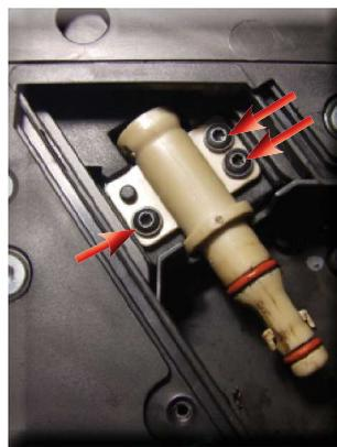
Loosen the screws as illustrated and remove the boiler pin.
