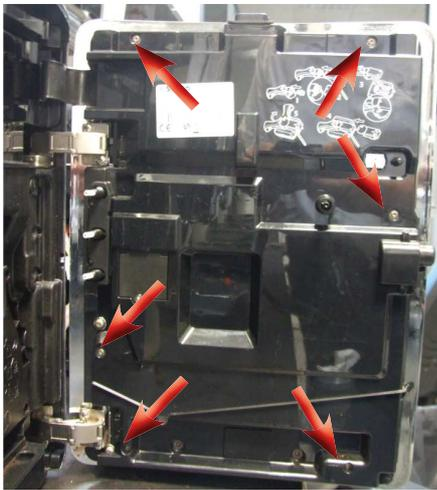
Loosen the screws as illustrated to remove the inner front panel cover
