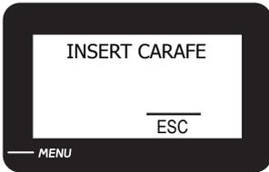
An operation that requires a dispensing cycle from the milk container has been selected. Insert the container and press the "esc" key to cancel the selection.
