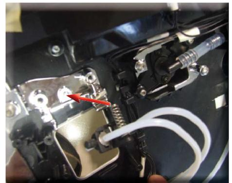
When replacing it, make sure you reposition the spring correctly
