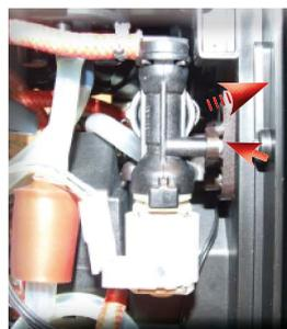
Loosen the screw as illustrated and remove the clip
