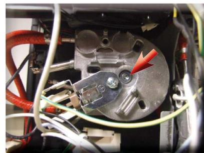
Loosen the screw as illustrated and disconnect the electrical and water circuit connections.
