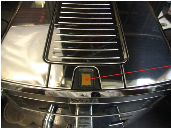
Digital ID (digital fingerprint identification device)
