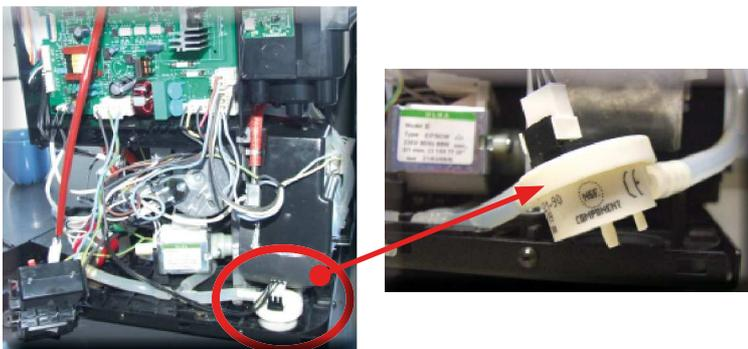
Lift the flow-meter out of the component mounting support and disconnect all electrical and water circuit connections.
