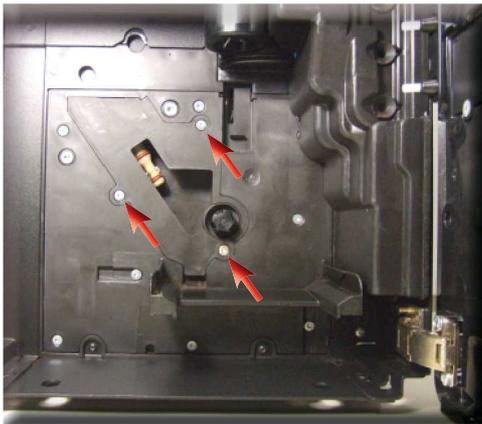
Loosen the screws as illustrated and remove the boiler pin.
