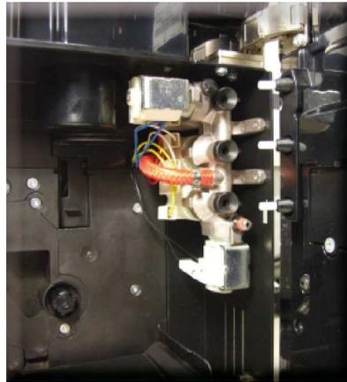
Loosen the screws as illustrated, making sure that the frothing valve does not fall and damage the connections.
