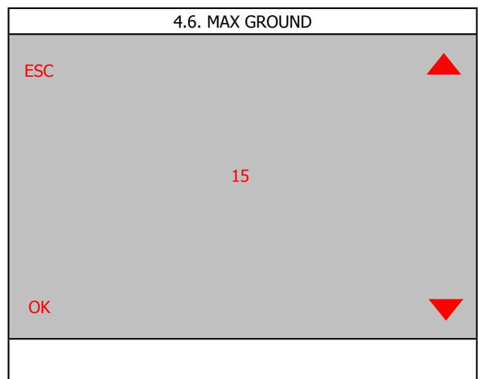
**MAX GROUND** (can be used to select the maximum number of coffee grounds batches . The range may be set between 10 and 20).
