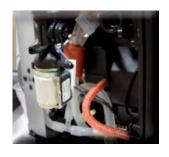
Disconnect the electrical and water circuit connections
