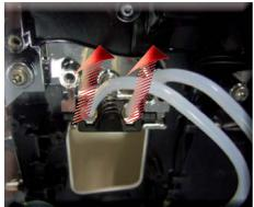
Remove the Teflon pipe support assembly
