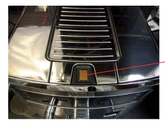
Digital ID (digital fingerprint identification device)
