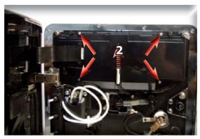
Slide the capacitive sensor out (1) along with the door presence reed sensor (2), loosen the screws highlighted and remove the CPU board cover.
