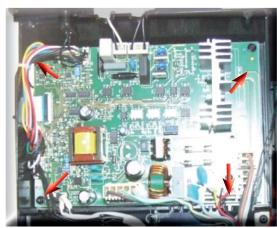
**2**) Loosen the screws as illustrated and remove all electrical connections.
