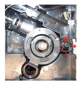
A technician will be able to adjust the grinding level even further, working directly on the coffee grinder by pressing and turning the ringnut (C) as illustrated. (clockwise + to increase the coffee grain size and anticlockwise - to decrease it)
