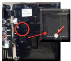
Loosen the screw as shown.
