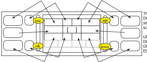
The 4 buttons (ESC, OK, UP and DOWN) highlighted in yellow, at the side of the display, can be used to scroll through the Test Mode:
