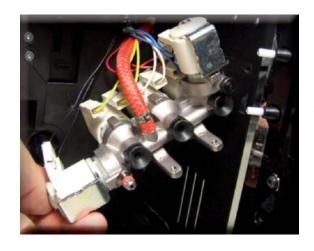
Disconnect all electrical and water circuit connections.
