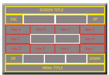
In Test Mode, all loads are initially deactivated. To activate a load, simply press the corresponding key on the keyboards at the side just once.
