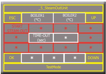
This screen corresponds to the steam\_out cycle, used to empty the coffee boiler and the hot water/steam boiler.
