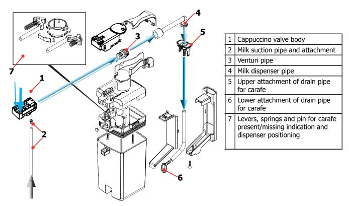
Functional method for the production of milk-based beverages and circuit cleaning When the solenoid valves open and let air or hot water/steam through, the following situations occur:
