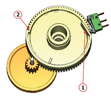
The gearmotor is powered by a direct current motor that engages with the smaller double toothed wheel using a worm screw. The brewing unit is mounted on the axle of the large gear wheel and when a coffee is requested, it moves from the home position to the dispensing position, and then back to the home position again.
