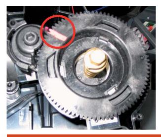
In the start position, both markings must be aligned.
