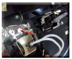
When replacing it, make sure you reposition the spring correctly
