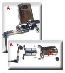
Remove the dispenser (photo B); when replacing it, make sure the spring highlighted is positioned correctly.
