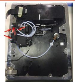
Remove the screws shown and pull the Teflon pipe support cover away from the carafe
