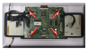
Loosen the screws as illustrated and remove all electrical connections.
