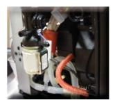
Disconnect the electrical and water circuit connections
