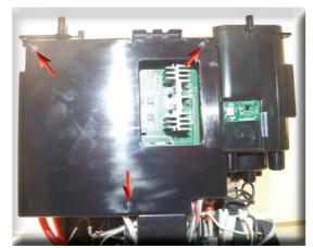
**1**) Loosen the screws as illustrated and remove the card cover.
