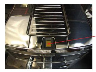
Digital ID (digital fingerprint identification device)
