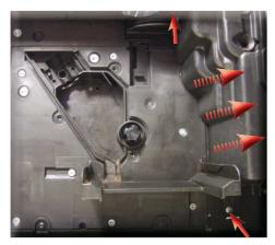
Loosen the screws as illustrated and remove the frothing valve protection.
