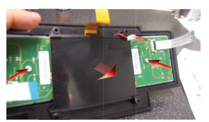
Remove the display support, loosen the screws highlighted and draw out the board, keys and the display.
