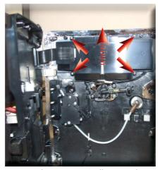
Loosen the screws as illustrated, slide out the door presence reed sensor and remove the CPU card cover.
