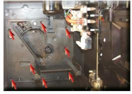
Loosen the screws as illustrated and remove the gearmotor cover.
