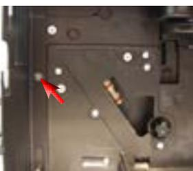
Unscrew the screws as indicated to reach the screw anchoring the multi-way valve to the support
