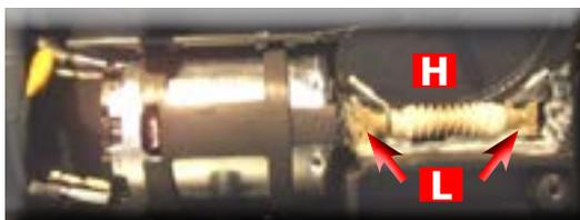
When replacing the motor and the transmission shaft, make sure the guide runners (L) are in the right position. Grease the shaft thoroughly and evenly.
