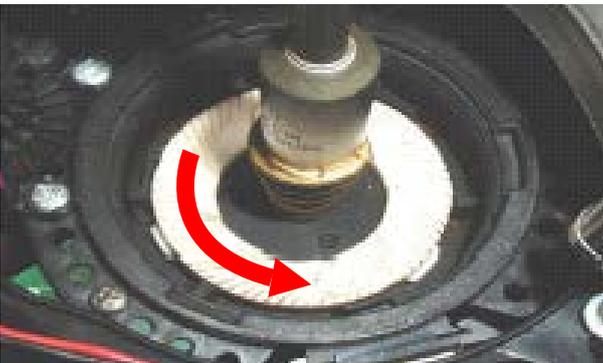
Turn the grinder blades anticlockwise out of the support.
