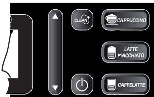
Flashing red LED. Machine in Stand-By "⏻"
