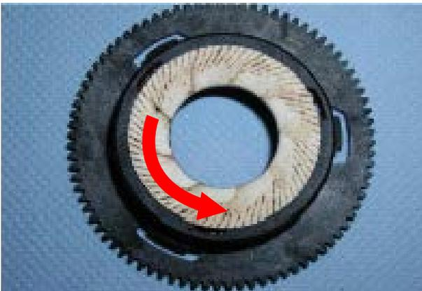
Turn the grinder blades clockwise out of the support. The bayonet connections can be accessed from the rear.
