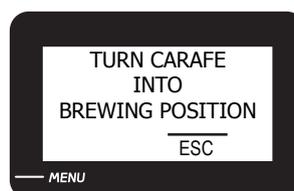
A beverage containing milk has been selected. The machine requires the carafe handle spout to be placed in the dispensing position. Press "ESC" to cancel the operation.
