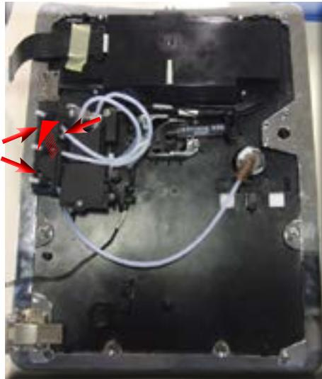
Remove the screws shown and pull the Teflon pipe support cover away from the carafe
