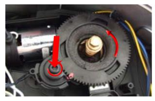
Press down on the grinder adjuster and then turn the upper grinder blades support anticlockwise until it stops.
