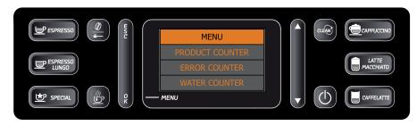
The entry to Diagnostics Mode shows a screen as seen in the figure at the side and pressing [IMG] allows to scroll through all menus present.
