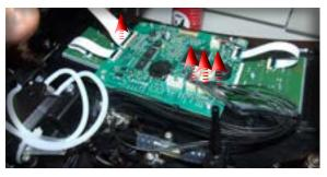
Remove the connections, loosen the screws highlighted and remove the board
