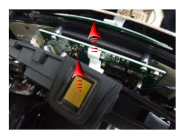
Remove the connection on the board and lift out the digital ID
