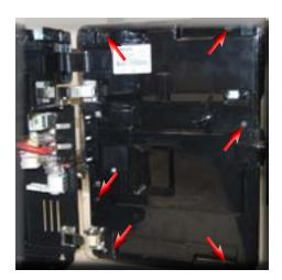
Loosen the screws as illustrated to remove the inner front panel cover.
