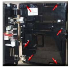
Loosen the screws as illustrated to remove the inner front panel cover.
