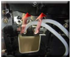
Remove the Teflon pipe support assembly
