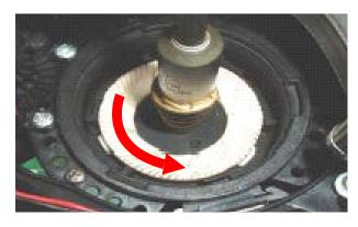
Turn the grinder blades anticlockwise out of the support.
