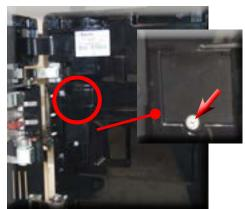
Loosen the screw as shown.
