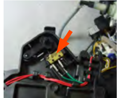
Lift the assembly and in the back there is the microswitch.
