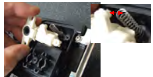
In the reassembling make sure the spring is repositioned correctly (see photo).
