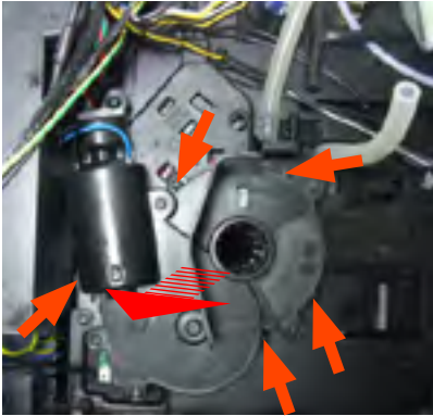
Loosen the screws highlighted and remove the gearmotor assembly.
