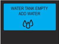
Remove the water tank and fill it. You can fill the water tank also through the dedicated hole on the lid.
