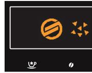
The machine needs to be descaled. Follow the steps described in the "Descaling" chapter of this manual. Please note that not descaling your machine will ultimately make it stop working properly. In this case repair is NOT covered under your warranty.
