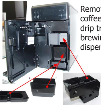
Remove the water tank, coffee container and cover, drip tray, dreg drawer, brewing unit, hot water dispenser, Milk carafe.
