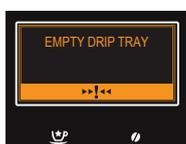
Open the service door and empty the internal drip tray.
