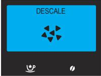
Machine descaling is needed. Refer to the maintenance menu to select and start the cycle.
