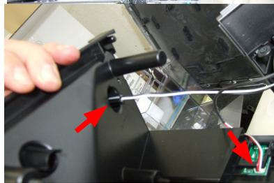
Disconnect the hydraulic and electrical connections highlighted
