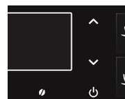
The red light flashes. Press any button to exit the stand-by mode.
