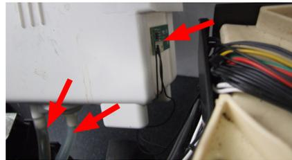
Disconnect all electrical and water circuit connections and remove the top cover.
