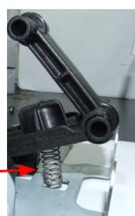
In the reassembling make sure the spring is repositioned correctly (see photo).
