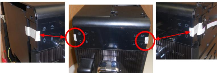
**CAUTION:** Every time that it's necessary to access inside the machine, after removing of the two lateral panel, the capacitive keyboard must be fixed on the appliance side with paper adhesive tape, as shown in the image.
