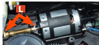
When replacing the motor and the transmission shaft, make sure the guide runners (L) are in the right position.
