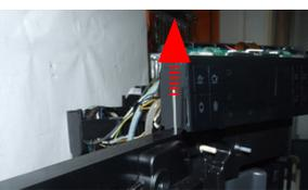
Lift the pin with a screwdriver and remove it through the top of the door.
