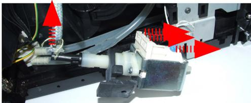
Disconnect the electrical / idraulics connections.
