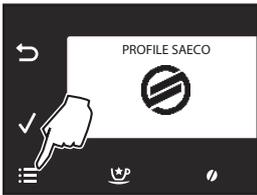
Press the "☰" button to access the machine main menu.
