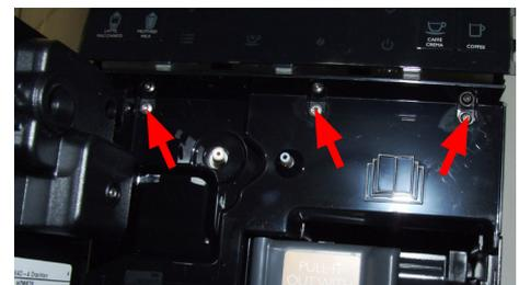
Remove the rubber plugs and unscrew the screws shown
