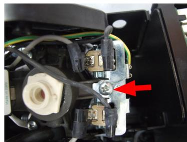
Loosen the screws highlighted and remove the thermostats unplugging from the electrical connections.
