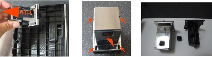
Remove the dispenser, remove the insert and unhook the anchors.
