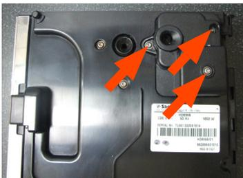
Unscrew the screws indicated and remove the cover.
