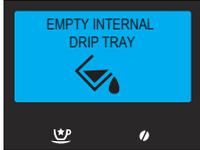
Open the service door and empty the internal drip tray.
