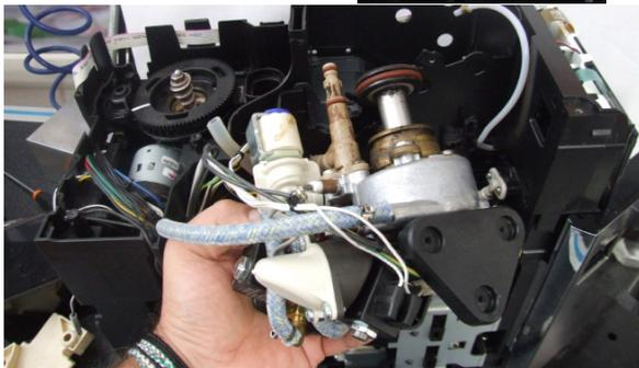
Remove the assembly and disconnect the electrical / idraulics connections.
