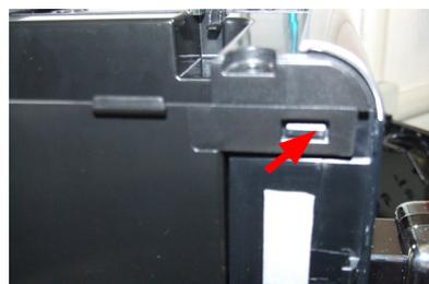
Press the parts highlighted and lift the top cover
