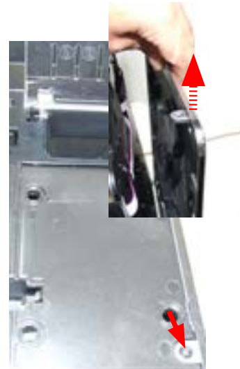
Remove the cup warning lid making sure to rise it near the hooks highlighted
