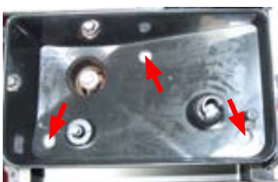
Remove the rubber plugs and unscrew the screws shown
