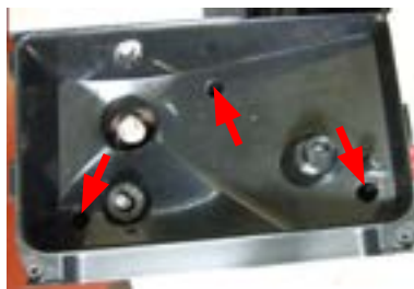
Remove the rubber plugs and unscrew the screws shown
