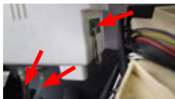
Disconnect all electrical and water circuit connections and remove the top cover.
