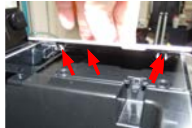
Remove the cup warning lid making sure to rise it near the hooks highlighted
