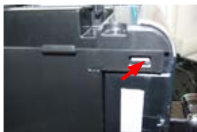
Remove the rubber plugs and unscrew the screws shown
