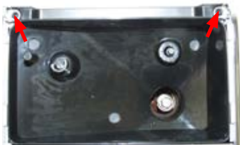
Unscrew the screws shown and remove the lateral panels
