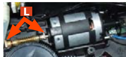
When replacing the motor and the transmission shaft, make sure the guide runners (L) are in the right position. Grease the shaft thoroughly and evenly.
