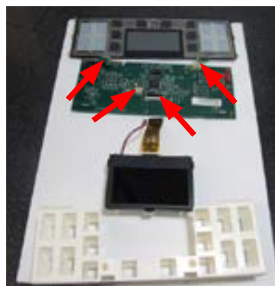
Disconnect the electrical connections.
