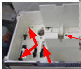
Unscrew the screws shown.
