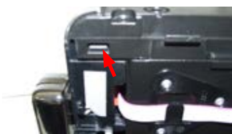
Remove the rubber plugs and unscrew the screws shown
