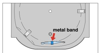
Note: Please make sure while re-assembling the new thermostat that the routing will be done as shown in below picture.
