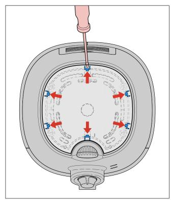
Use a crosshead screw driver to unscrew the 4 screws A.
