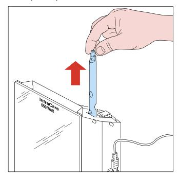
4. Remove the other lamp holder and unplug the wires.
